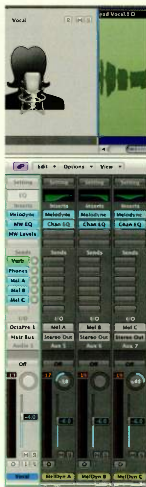
FIG. 1: The pitch-corrected vocal is sent to three buses, each with an instance of Melodyne Editor with different pitch and timing deviations. The channel strips have separate panning and EQ.
