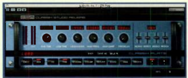
FIG. 3: IK Multimedia's Classik Studio Reverb resembles the front panel of an outboard reverb unit and provides two complementary editing modes, Easy and Advanced.
