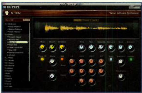
FIG. 4: VirSyn's Reflect uses convolution technology for some of its programs, combining up to 200ms of an impulse response with an algorithmic tail.
