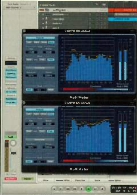
FIG. 2: It's useful to have two multimeter plug-ins active: one at the beginning of the chain and one at the end.
