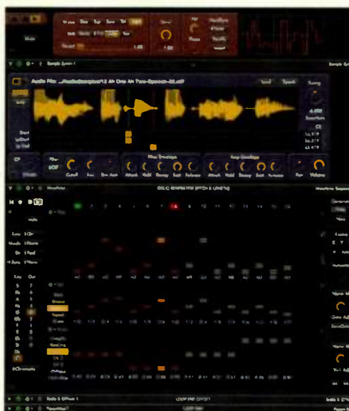
FIG. 1: This Numerology Stack uses an LFO (top) and a CV lane of a MonoNote sequencer (bottom) to modulate the sample start and loop boundaries of the speech clip in the Sample Synth module (middle). The MonoNote also sets the playback pitches and step lengths.
