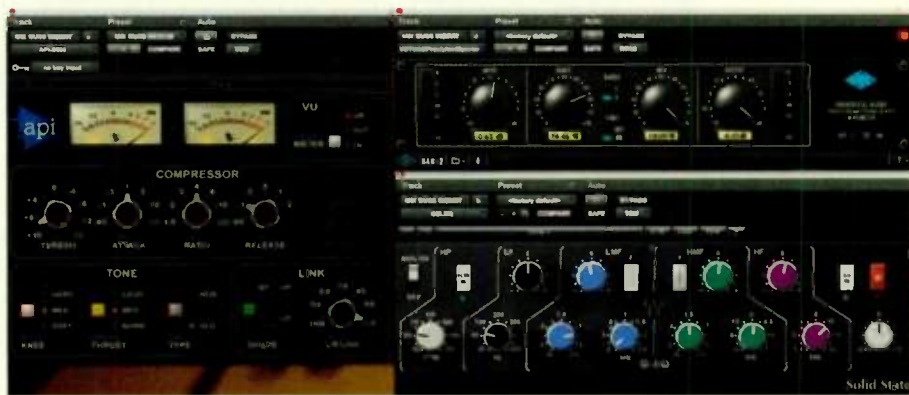
FIG. 2: Start the mix with a compressor, a brickwall limiter, and an EQ plug-in on the mix bus insert track.
