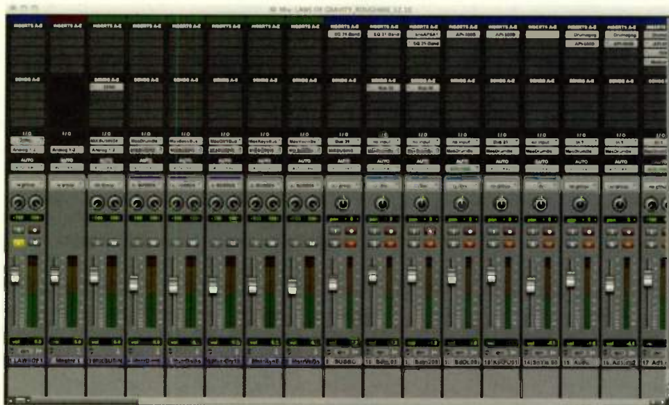
FIG. 1: Assign the drums, keys, guitars, and vocals to subgroups, and route all the subs through the mix bus insert track.
