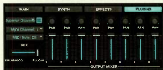
Figure 3: Drumagog's plug-ins section can load any VSTi plug-in you own for direct triggering. The output mixer includes level and pan controls for the hosted plug-in's multiple outputs (if the VSTi includes these).
