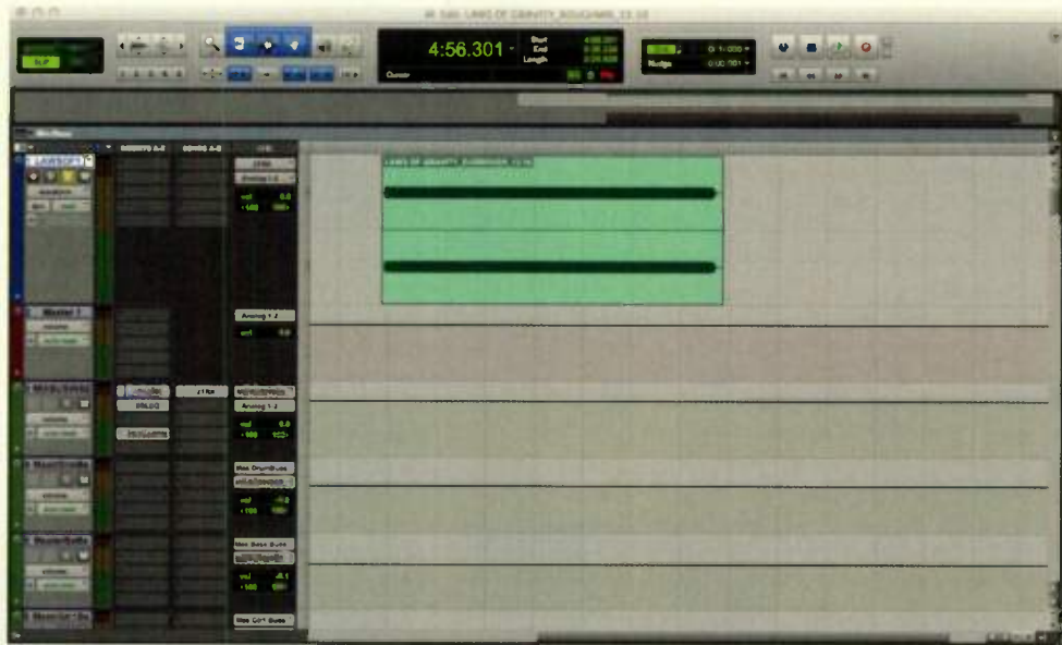
FIG 3: Printing to a track in the session keeps your mix inside the session, making later retrieval easier.
