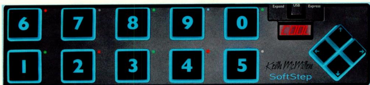
FIG. 1: KMI SoftStep's bank of ten Keys can send independent streams MIDI or OSC data from each pedal.
