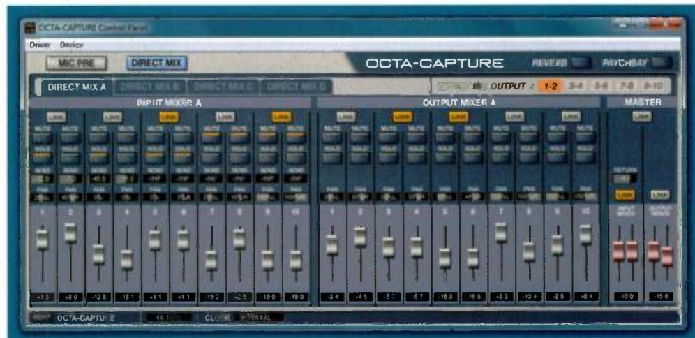
Fig. 3 The Octa-Capture offers a flexible monitoring system called Direct Mixer that combines zero-latency input monitoring with DAW-playback tracks.
