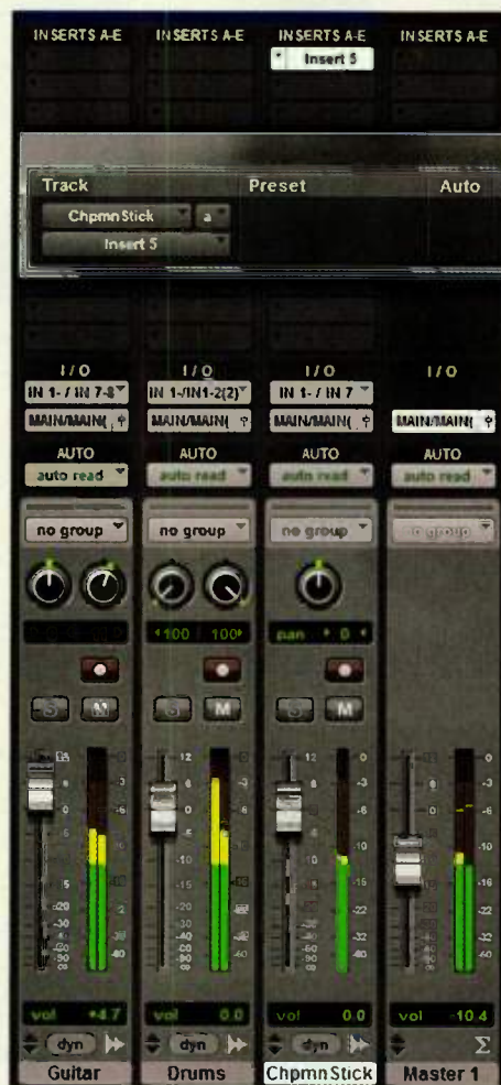
Fig. 1 Pro Tools makes it easy to add external hardware: Choose an insert, and tell it which buses you want to use as audio I/O. In this screen shot, a Chapman Stick track is being fed through a Line 6 PODxt via I/O bus 5.
