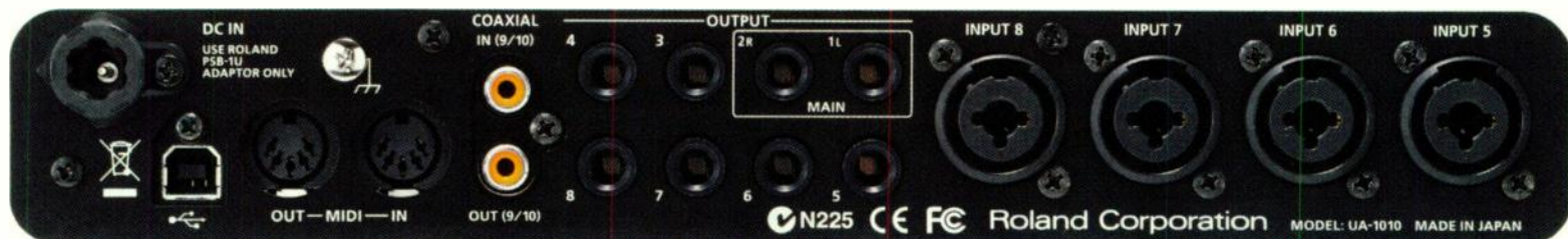
Fig. 1 The rear panel includes eight 1/4-inch outputs, stereo S/PDIF I/O, and MIDI I/O.
