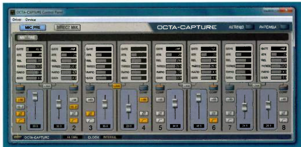
Fig. 2 Each input channel on the Octa-Capture is configurable with respect to sensitivity, phantom power, phase invert, impedance (channels 1 and 2), low-cut, and compression.
