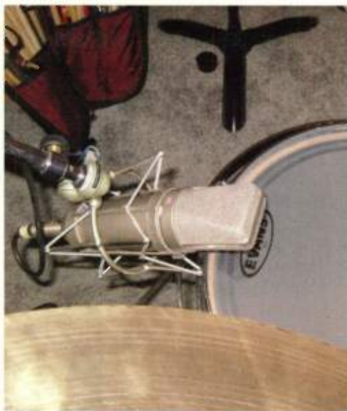
Fig. 2 In this overhead view, a Neumann U87a multi-pattern condenser, set to bi-directional mode, is placed on a floor tom. One of the mic's null points faces the ride cymbal in order to reject its sound.
