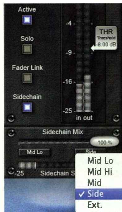
Fig. 2 The Sidechain Mix slider adjusts the relative balance of two sidechain signals. The thin vertical line of “LEDs” between input and output meters indicates the combined signals’ level in a keyed channel’s sidechain (with the Sidechain button activated).
