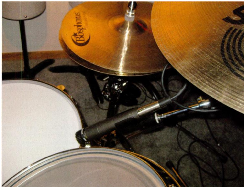
Fig. 1 A Shure SM57 cardioid mic is threaded between the hi-hat and high rack tom to record the snare drum. The hi-hat's sound is partially rejected by the 57's null point.
