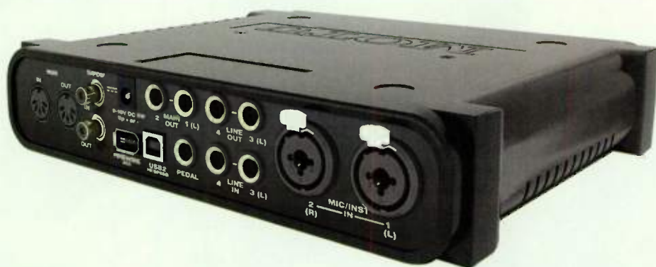
The two combo input connectors on MOTU's Audio Express can accommodate mics or instruments.
