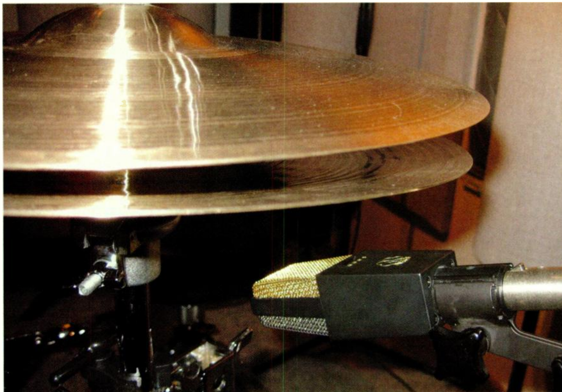
Fig. 1 An AKG C 414 B-TL II multi-pattern condenser mic is set to figure-8 mode and placed under the hi-hat. Its null point is aimed toward the snare drum in order to reject its sound.
