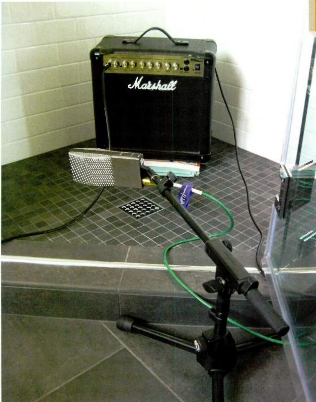
Fig. 1 An amp recorded in a tile-and-glass shower benefits from extra color provided by early reflections.
