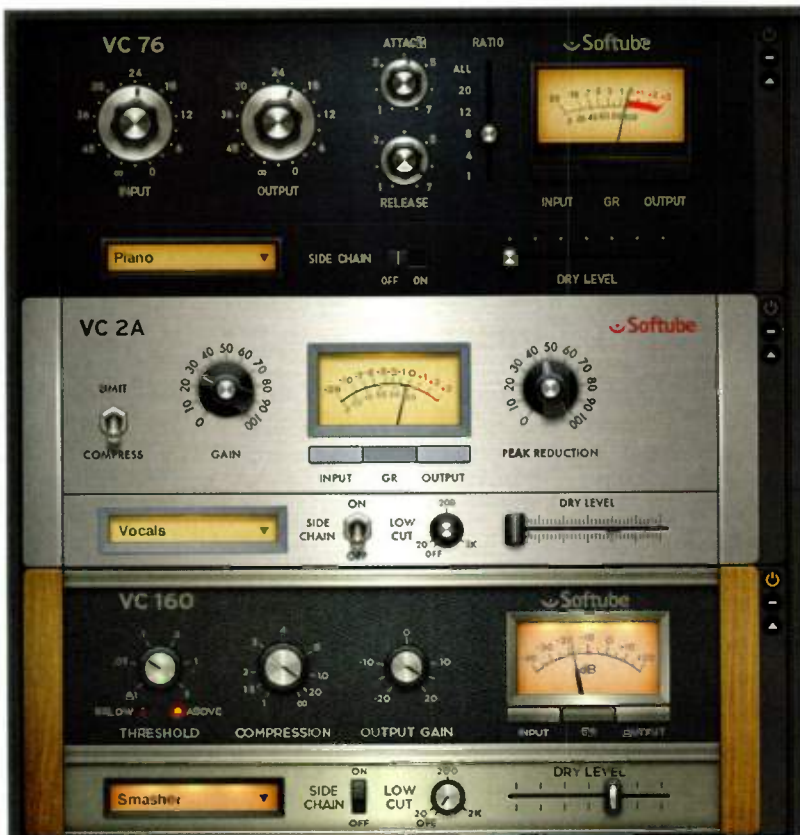
From top to bottom: The VC 76, VC 2A, and VC 160, each with their expansion panels open, showing the sidechain and wet/dry level controls.
