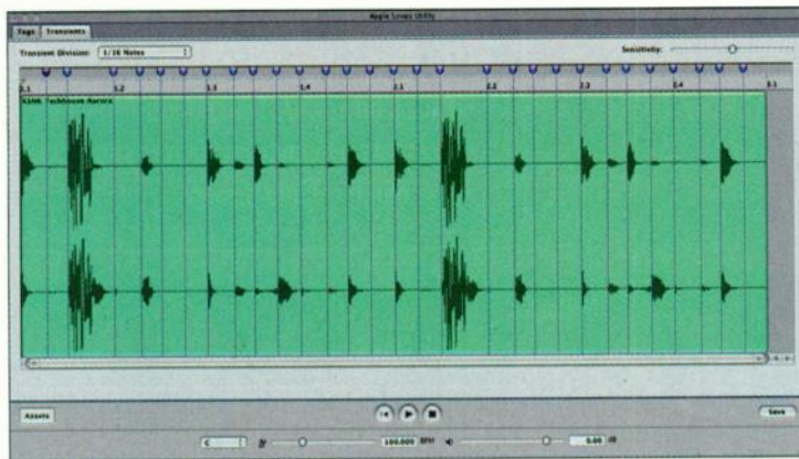
Fig. 3. The Apple Loops Utility is a free program that allows optimizing the stretching characteristics of AIFF or WAV files, as well as tagging them for database retrieval.
