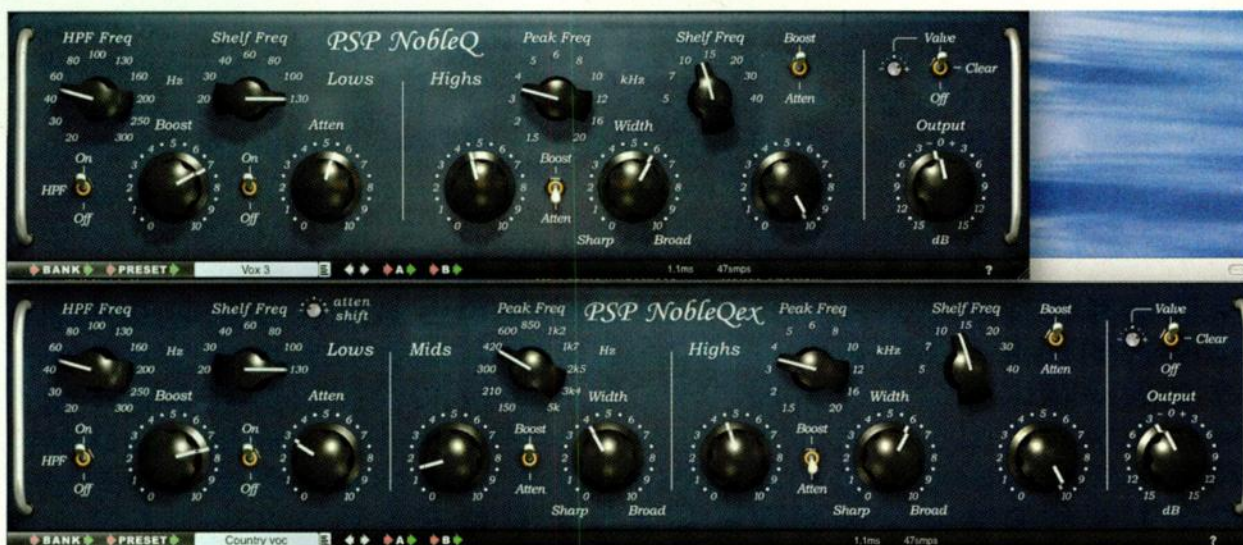
The PSP NobleQ (top) and NobleQex (bottom) plug-ins add vastly expanded capabilities to a classic passive-equalizer design.
