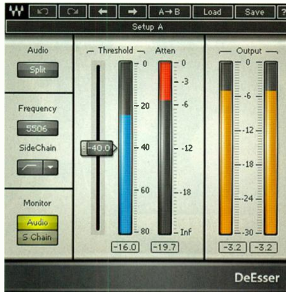
Fig. 2. Waves DeEsser dynamically softens high-frequency transients to take the edge off guitar-amp sims.
