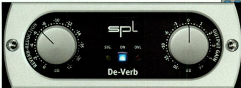
Fig. 3 Raise the Reverb-Reduction control on the SPL De-Verb plug-in to reduce reverb on any mono or stereo track.
