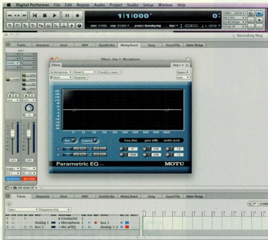
Fig 1. Plug-in routing for recording, using MOTU Digital Performer as an example.
