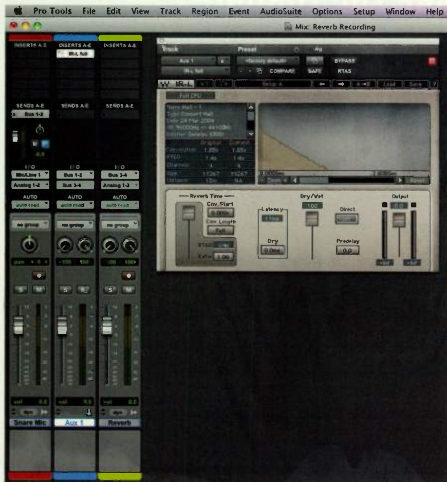
Fig 2. Recording an effect to a separate track.
