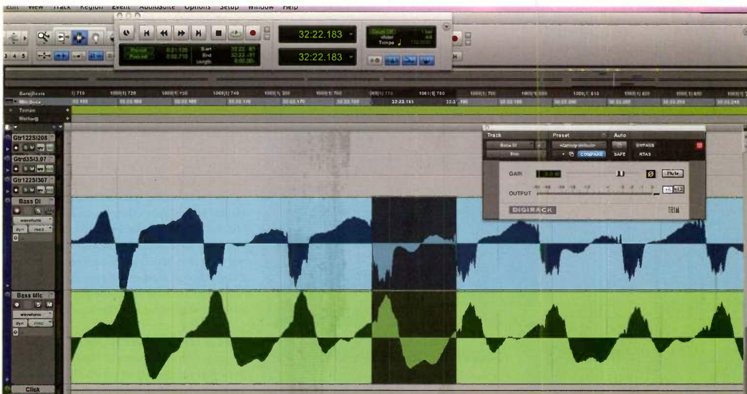
Fig. 2. A Pro Tools session with a bass DI track and a bass mic track. In the highlighted area, note that when the waveform in the DI track goes negative, the waveform in the mic track moves positive. This opposition in signal polarity will cause weak bass when the tracks are added together. The solution is a trim plug-in (shown), with the polarity reversed (yellow 0 indicator).
