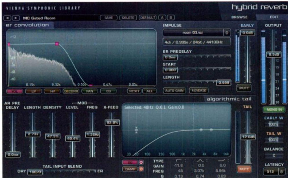
Fig. 1. Hybrid Reverb combines convolution reverb in series and parallel with algorithmic reverb. This shows the author's setup for gated-room reverb.
