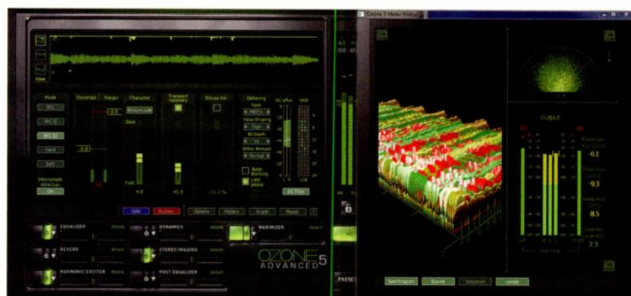
iZotope Ozone5 Advanced’s main window, on the left, shows the Maximizer. Note the waveform along the top; the upper line shows gain reduction. The window on the right is the meter bridge. The spectrogram shows where the vocal (red) sits in the mixed output (green). Drums are yellow and tan.
