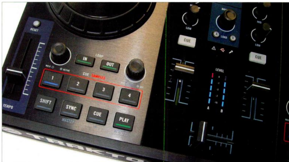
Fig. 2. Part of NI's S2 controller, which is optimized for Traktor. The controls for one deck are in the lower left, with the platter above it. Faders for the two decks, meters, and the crossfader are to the right. The deck 2, effects controls, and most common controls are not shown.
