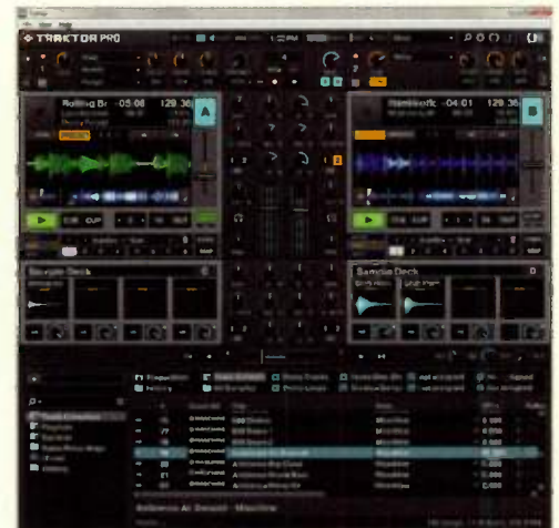
Fig 3. Traktor Pro 2 maps much of what you see to the hardware controls in NI's S2 (and other NI controllers, as well as some Traktor-specific controllers made by other manufacturers such as Numark). The two virtual decks are outlined in gray, with common controls toward the middle and a browser along the bottom.
