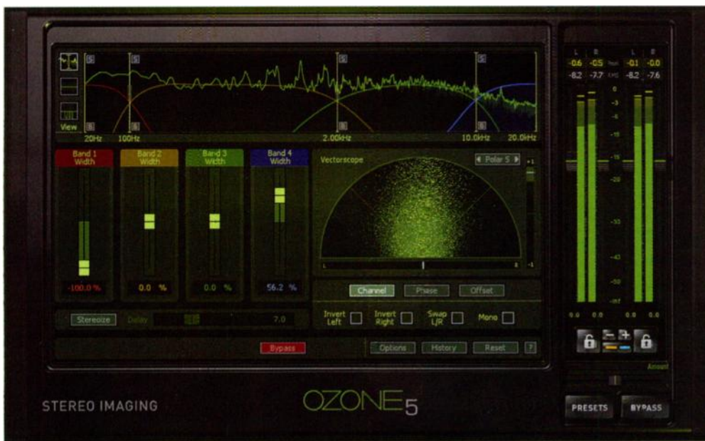
Fig. 4. Ozone 5 Advanced's multiband Stereo Imaging plug-in is an excellent tool for widening your mix's soundstage. Here, frequencies below 100Hz are narrowed to mono while highs above 10kHz are widened.
