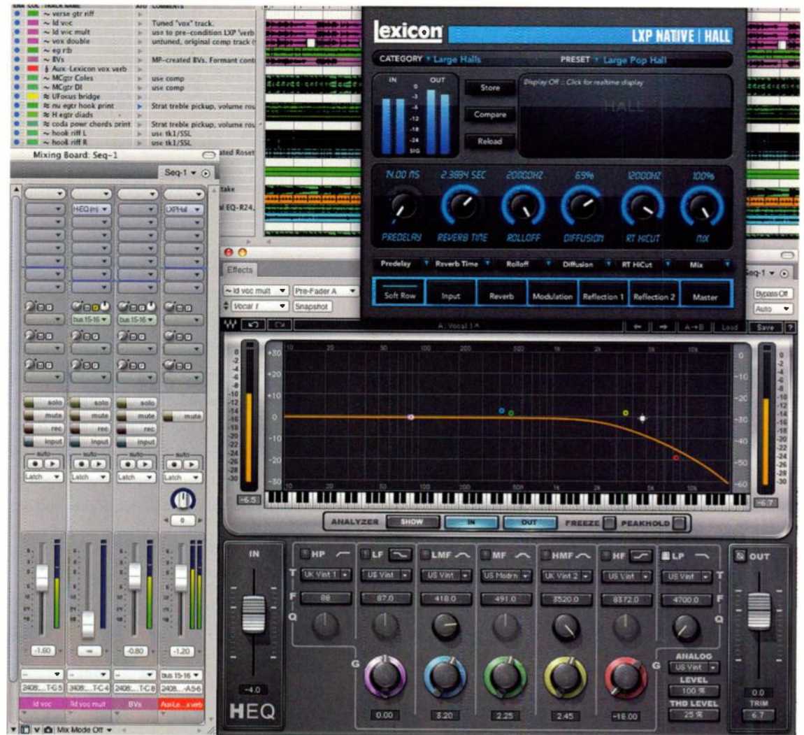
Fig. 1. A mult for a lead vocal track is removed from the mix bus and sent pre-fader to a Lexicon LXP Native Reverb plug-in in Digital Performer. The Waves H-EQ Hybrid Equalizer plug-in pre-conditions the mult's reverb send, rolling off highs.
