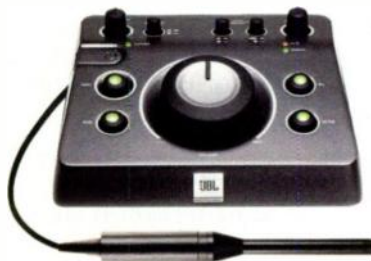
Fig. 3. JBL's MSC-1 is an accessory device that, after being calibrated with a computer, corrects for acoustical problems at lower frequencies.
