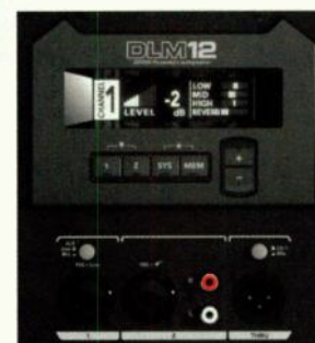
Fig. 2. DLM12 control panel (same as DLM8).
