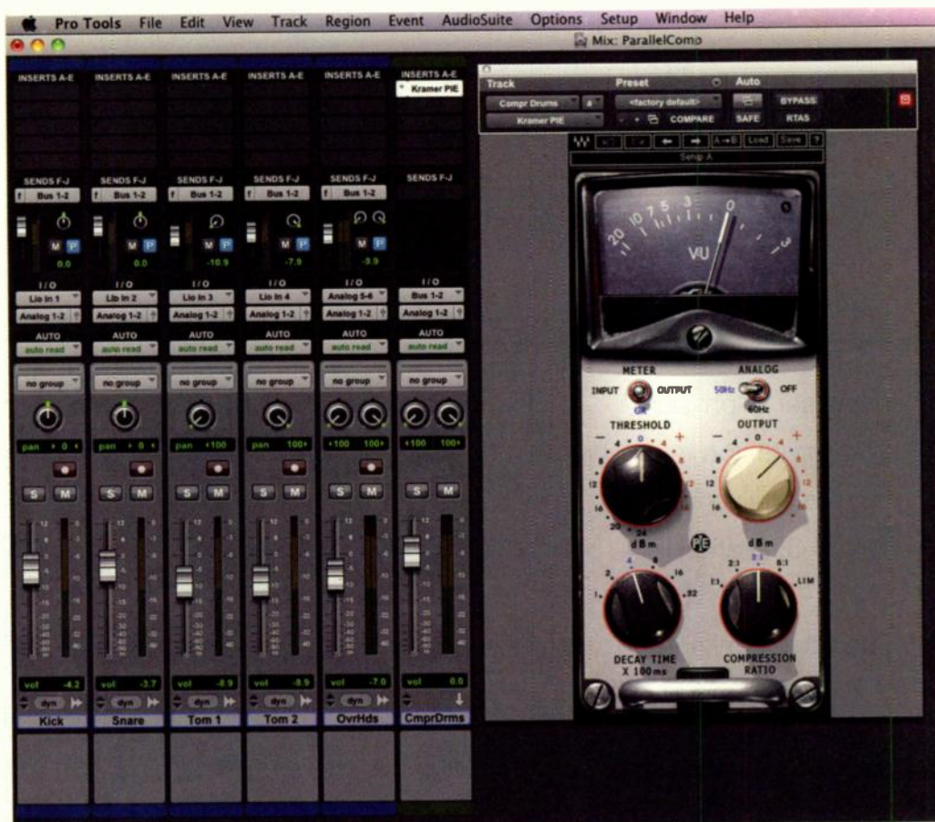
Fig. 1. This screenshot shows parallel compression applied to drum tracks in Pro Tools. Sends are used to route the drum tracks to an Aux track labeled "CmprDrms" (Compressed Drums). This track has a compressor (Kramer PIE) plug-in inserted, creating a new compressed version of the drums which is mixed in with the original drum sounds for a unique effect.
