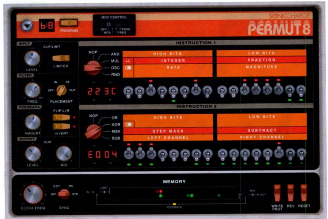
Sonic Charge Permut8 uses two versatile digital instructions to read from the audio memory buffer.
