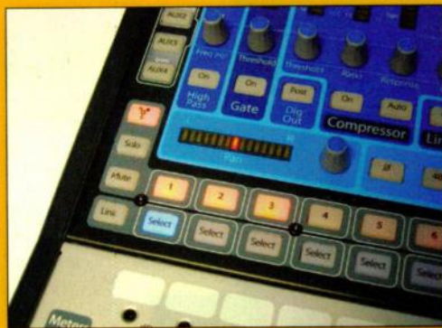
Fig. 2. This shows the FireWire button enabled in PreSonus's StudioLive 16.0.2 mixer; inputs 1-3 are set to inputs coming in from FireWire instead of their analog inputs.
