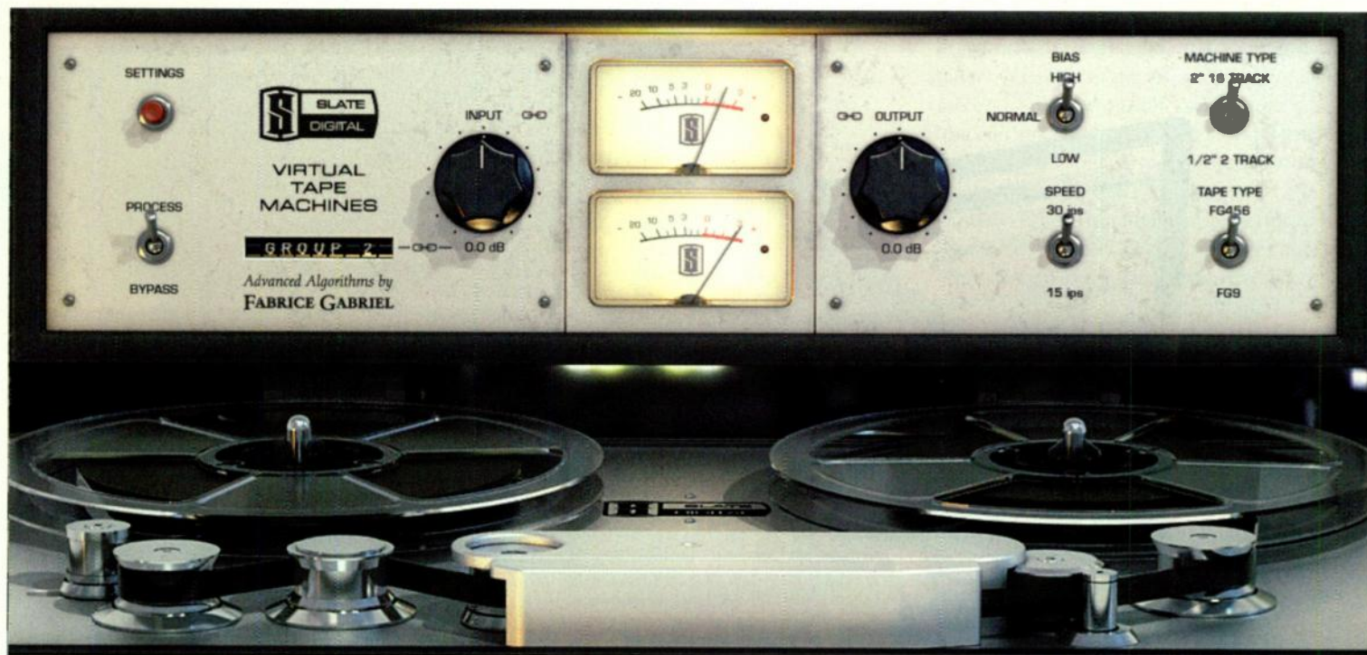
Fig. 1. Virtual Tape Machines emulates two tape decks, each using alternate tape formulations and operating at different speeds.
