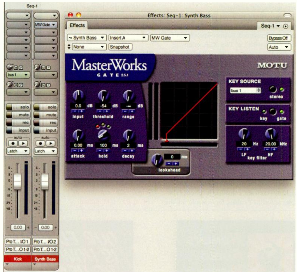
Fig. 1. The MasterWorks Gate plug-in from Digital Performer. The gate is inserted on the synth bass track; on the kick drum track, an aux send is routed to Bus 1. Bus 1 is then used as the gate's "KeySource."
