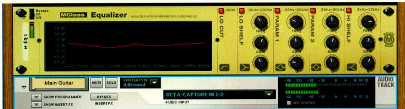
Reason's MClass Equalizer isn't just for mastering; it can handle most corrective EQ needs for guitar. Note that the 20Hz Lo Cut filter is enabled to get rid of "mud" below the guitar's range.
