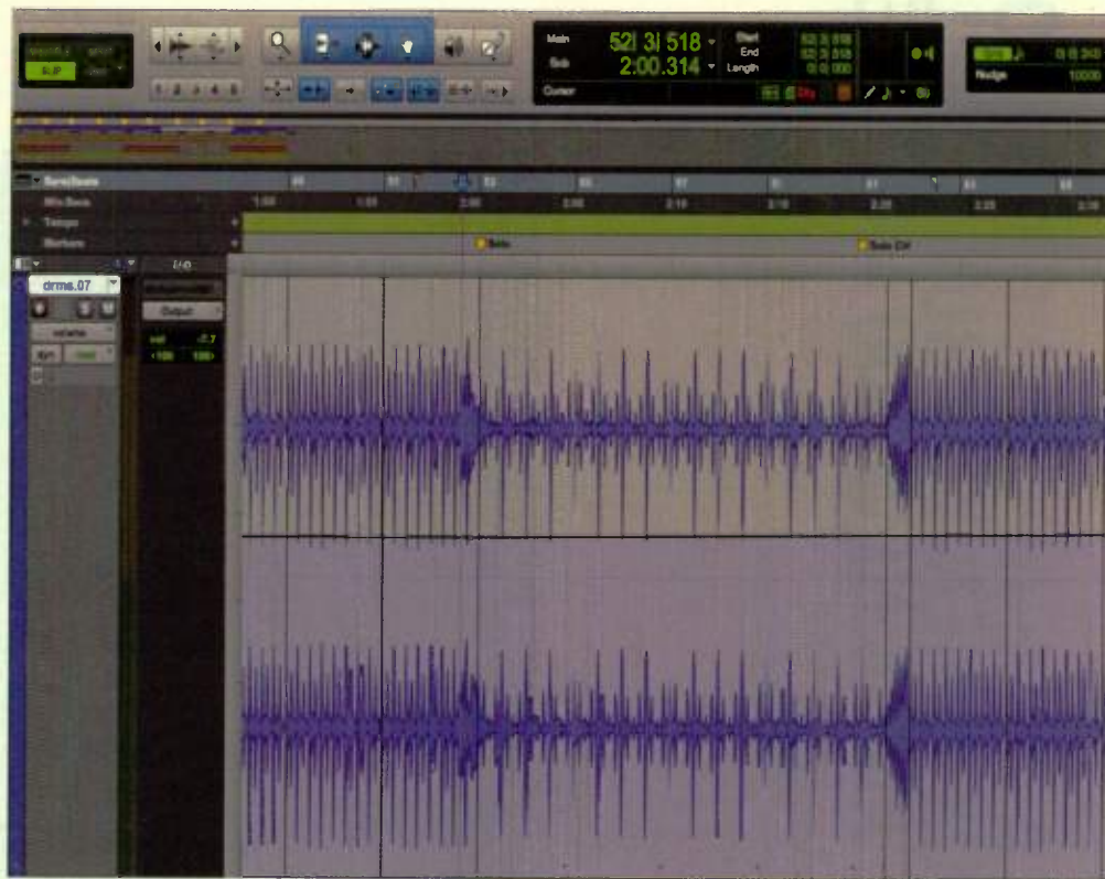
Fig. 2. Volume automation is used here to draw in a subtle rise in volume on the drum track during the solo section, to add to the dynamic interest.
