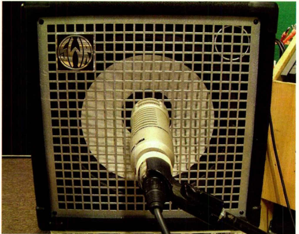
Fig. 6. Close, on-axis miking tends to give the “roundest” sound when miking a bass amp.
