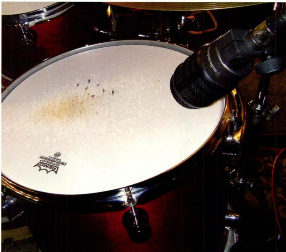
Fig. 4. With toms, it’s particularly important to place the mic where it won’t get hit by an errant stick.
