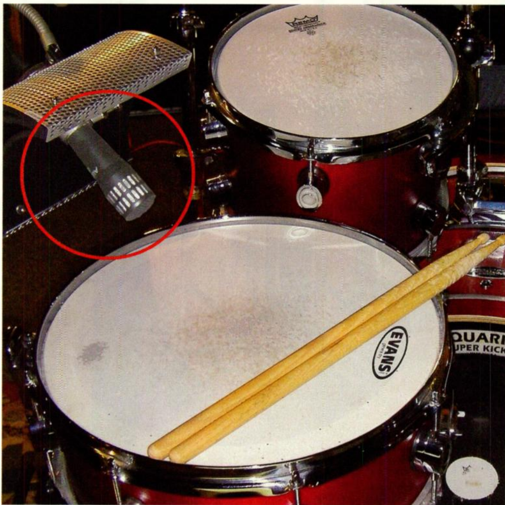
Fig. 2. When placing the snare mic, aim it at the snare's center, but also try placing it a bit off-center before making a final decision.
