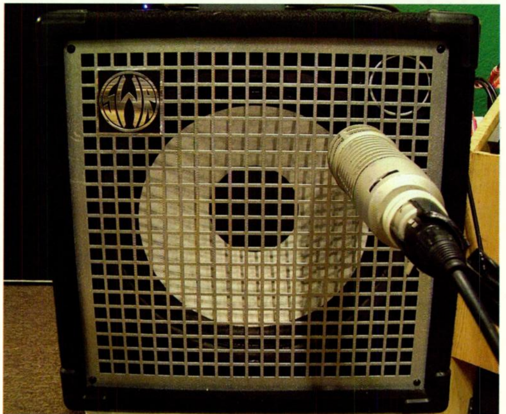
Fig. 7. Off-axis miking can yield a tighter sound, but here, it’s also being used to pick up the sound from the amp’s tweeter.
