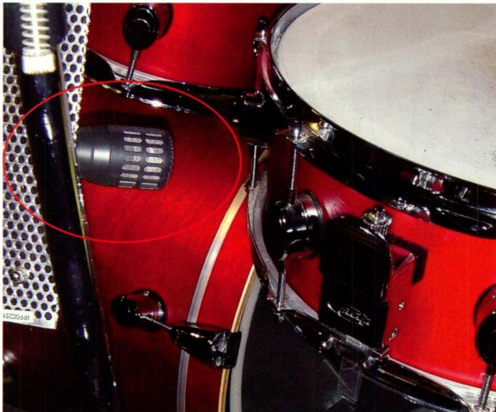
Fig. 3. The “side capture” option isn’t always about the sound—if the drummer has sketchy stick control, it can save your mic by taking the hit.
