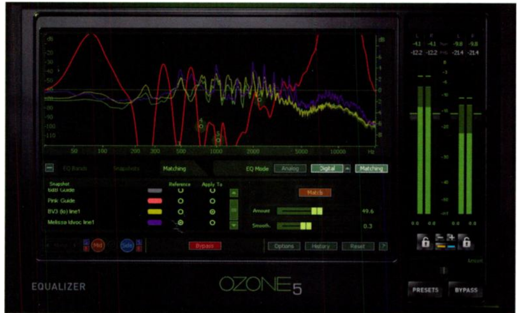
Fig. 1. The Equalizer plug-in in Ozone 5 Advanced applies matching EQ to a pitch-shifted vocal. Note the severe EQ (the off-the-scale red line in the top section of the GUI) needed to correct comb filtering and roll-offs caused by pitch shifting.
