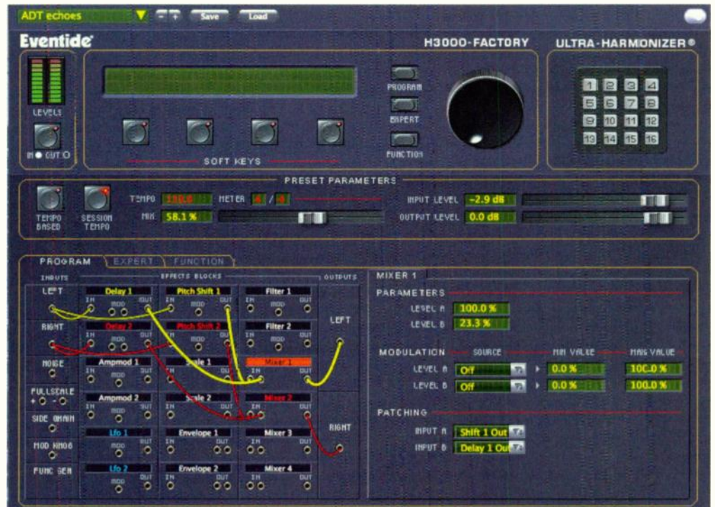
Fig. 1. H3000 Factory's signal flow is sequenced by dragging virtual patch cables in the GUI's lower-left section. Parameters for the currently selected block are accessed in the lower-right section. In this example, Pitch Shift 1's level is set to 100% and Delay 1's level to 23.3% in the summing mixer for the plug-in's left channel.
