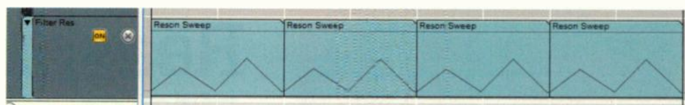
Fig. 3. Using track automation clips rather than CV signals will produce identical results, but more editing will likely be needed. Here, the filter resonance of a Subtractor is being swept repeatedly by identical two-measure automation clips to produce an LFO-like effect.
