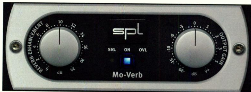
Fig. 2. SPL Mo-Verb can magnify the amount of natural reverb on a mono or stereo track to an extraordinary degree.
