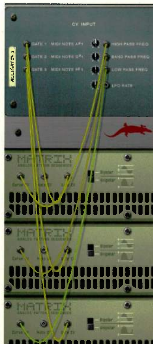
Fig. 7. To program your own patterns for the Alligator, hook up three Matrix sequencers as shown.
