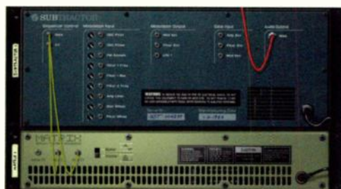
Fig. 2. The default routing of the Matrix Note and Gate CV outputs to the Sequencer Control inputs on a Subtractor. The unipolar/bipolar switch on the Matrix affects only the Curve CV output.
