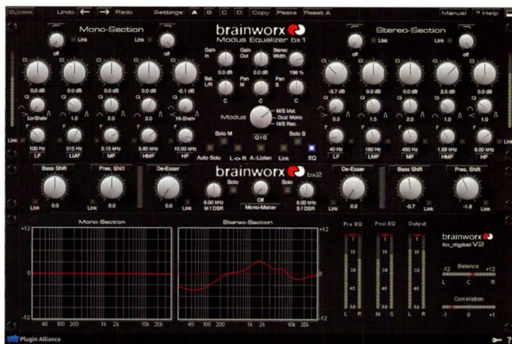
Fig. 3. Brainworx bx_digital V2 equalizes room tone on a stereo track, removing mud and attenuating sizzling frequencies, while simultaneously widening the soundstage.
