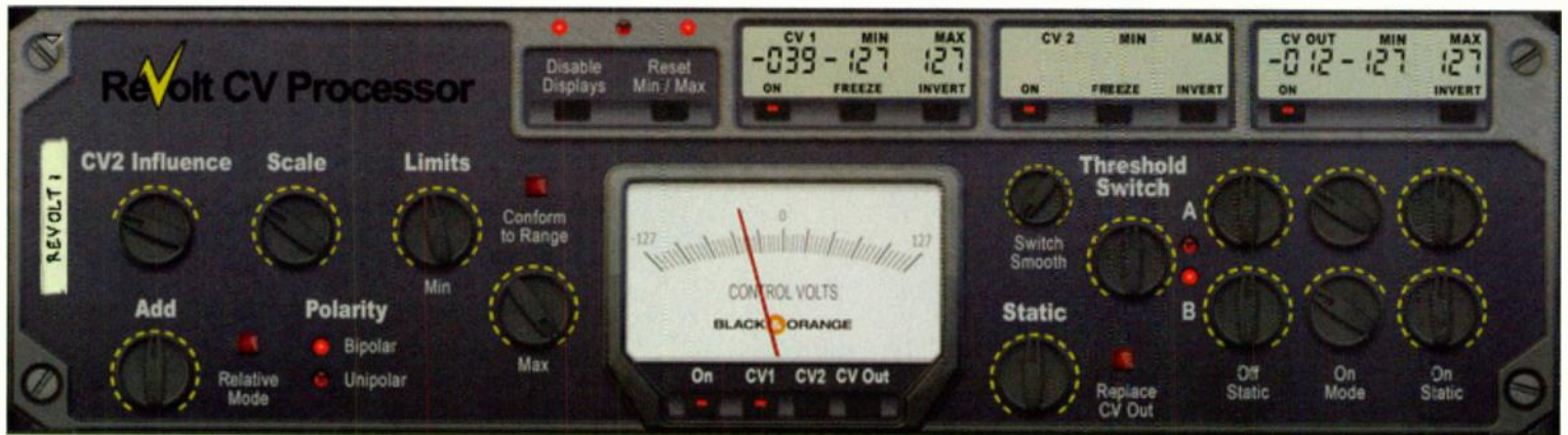
Fig. 8. The ReVolt CV Processor is an optional add-on. It has handy front-panel data displays and more than 20 CV connections on the rear panel.
