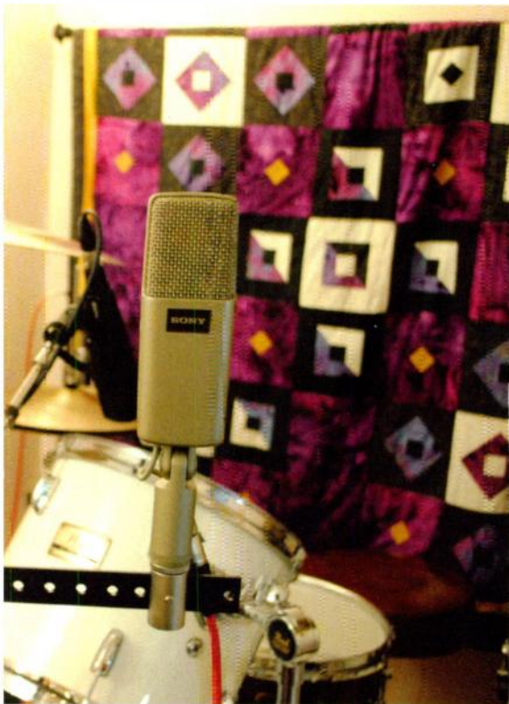
Fig. 5. Sony C48 multipattern mics set to omnidirectional and arrayed as a spaced pair.
