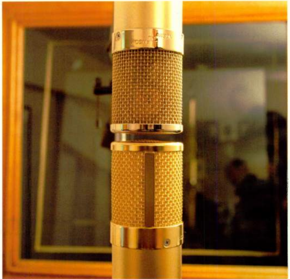
Fig. 1. This photo shows two microphones placed for Mid/Side Stereo. The bottom microphone is a Lawson L47 MP set to figure-eight and facing the side walls of the studio. The top mic is a Lawson L47 (cardioid-only) and is directly facing the source.
