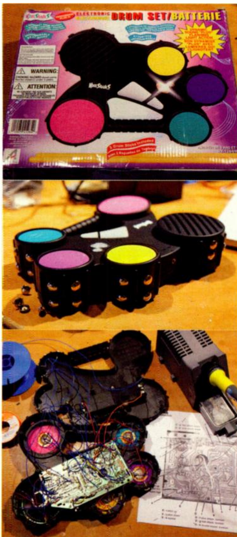
The KoolShades drum toy is a very lively body-contact bend. Note the upholstery tags used for the body-contacts and the mark sheet.
