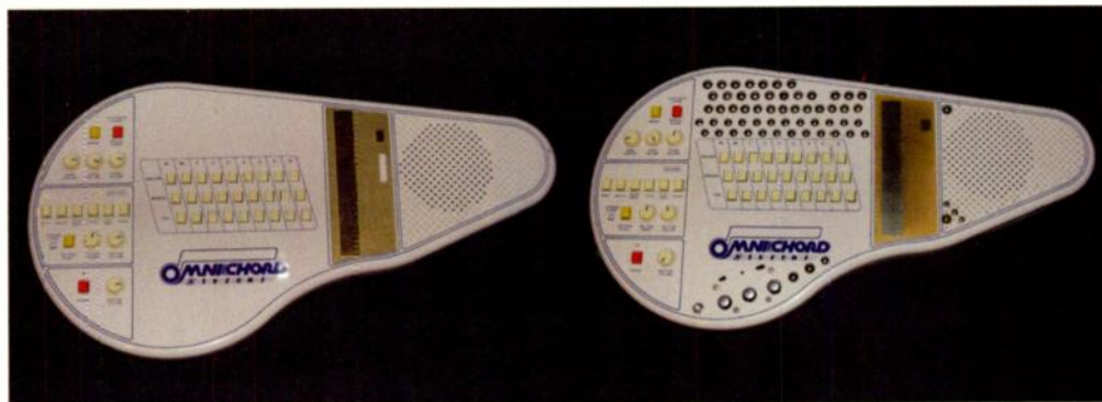
The Suzuki Omnichord OM-27 before and after bending. The three silver knobs on the lower side belong to a Ibanez DE-7 delay.
