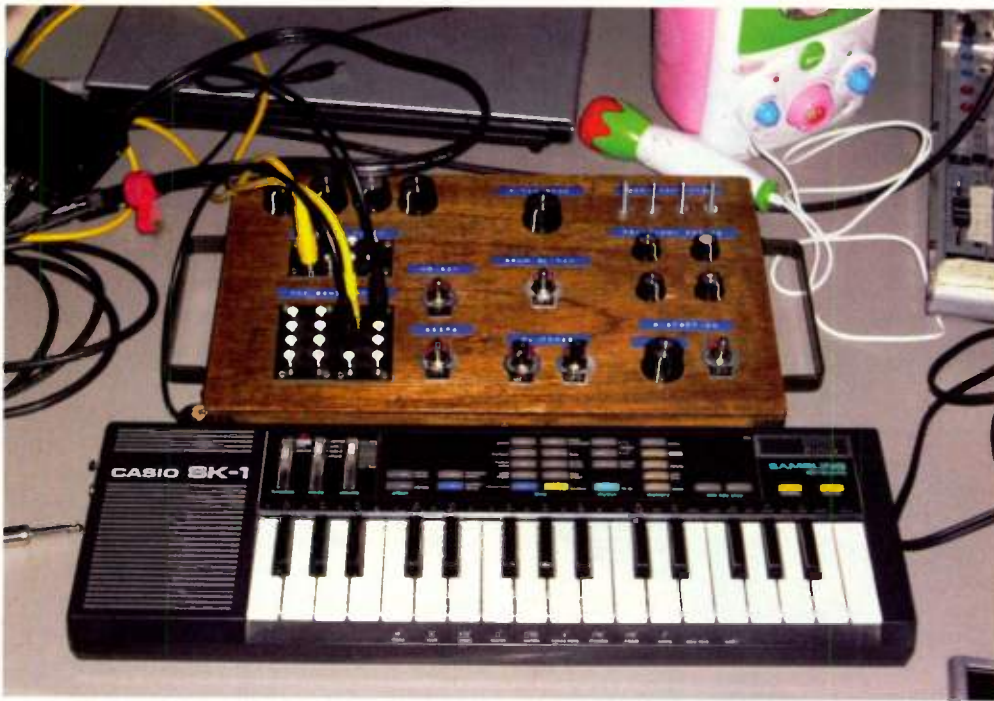
The Casio SK-1 is one of the best-documented and explored bending targets, with a wealth of great bends and a stable and reproducible behavior. This model is enhanced with a breakout box for the additional components.
