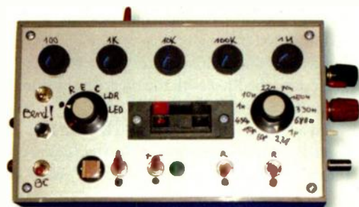
The KoolShades drum toy is a very lively body-contact bend. Note the upholstery tags used for the body-contacts and the mark sheet.
