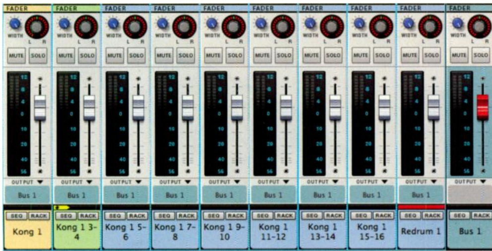
Fig. 2. To build a submix in Reason 7, pick the channels you want to include and select New Output Bus in the Edit menu. The selected channels will be routed automatically to the new destination.
