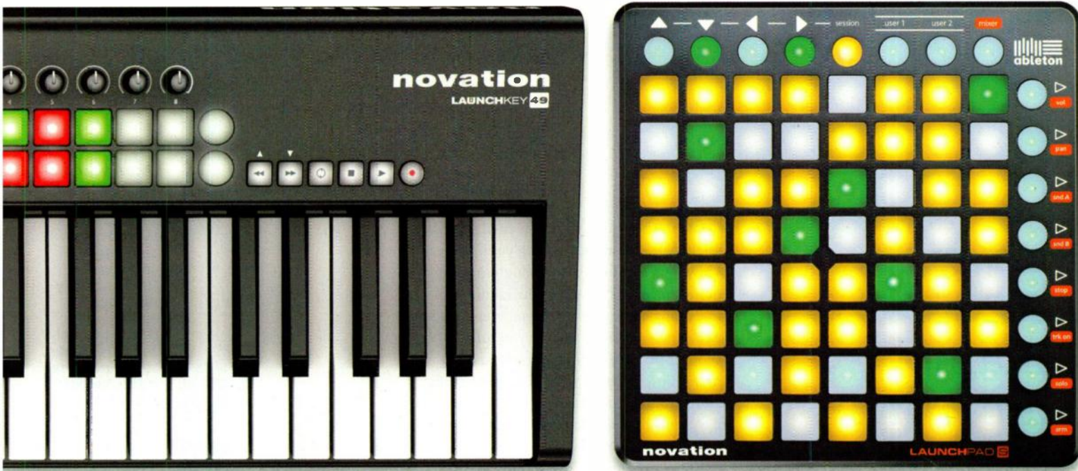
Fig. 2. The Launchpad S is faster and brighter than the original model, and it is MIDI Class Compliant.
