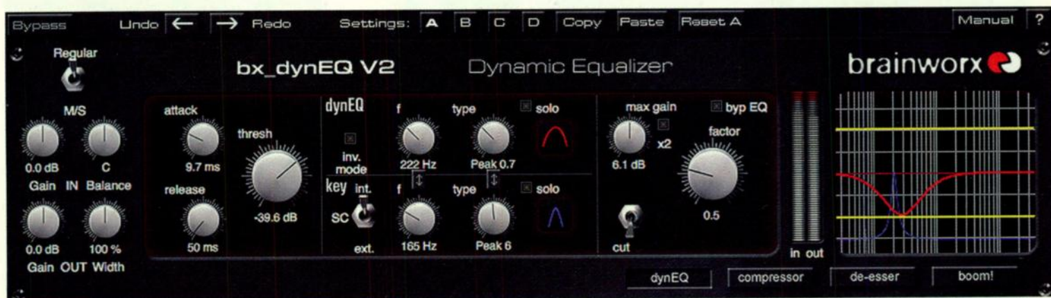
Fig. 1. The Brainworx bx_dynEQ V2 dynamic equalizer plug-in de-booms an acoustic guitar by cutting at 222Hz whenever an E note is played at the 2nd fret on the instrument's 4th string.
