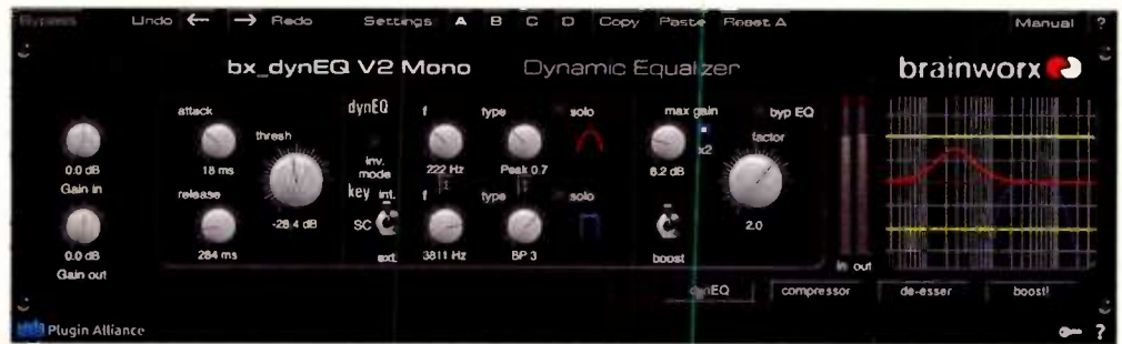
Fig. 3. bx_dynEQ V2 automatically boosts 222Hz when a solo violin plays very high notes, fattening the tone.
