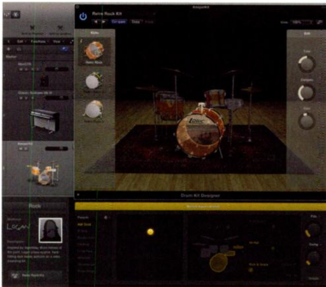
Fig. 1. A view of the Drum Kit Designer plug-in with the Drummer editor below it. The yellow ball in the editor's X/Y matrix adjusts the dynamics and complexity of the virtual drummer's performance.
