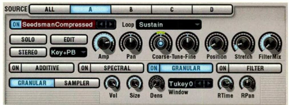
Fig. 1. Each of Camel Audio Alchemy's four oscillators can perform granular synthesis. The relevant parameters for granular control are the Position and Stretch knobs in the top row; the Size, Dens (density), RTIME (random time amount), and RPAN (random panning amount) knobs in the bottom row; and the Window drop-down.
