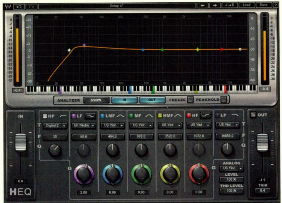
Fig. 1. Shelving and highpass filters are used at once in the Waves H-EQ Hybrid Equalizer plug-in to shape a bass guitar's sound.
