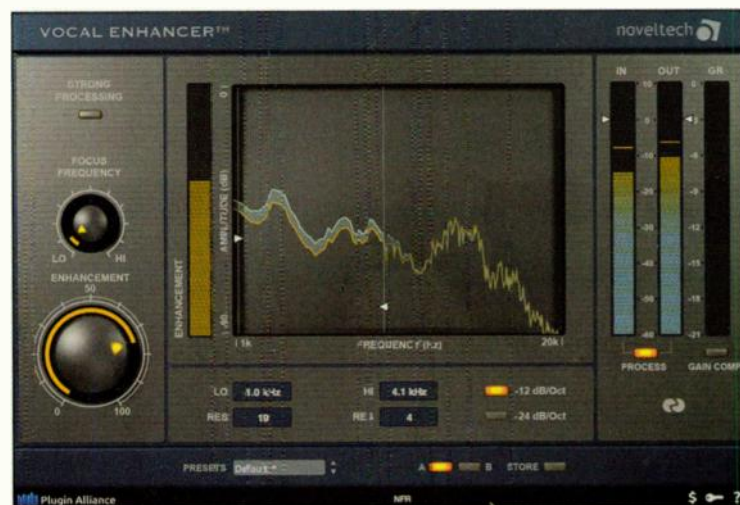
Fig. 2. Frequencies between 1Hz and 4.1kHz are dynamically enhanced to clarify a vocal track.
