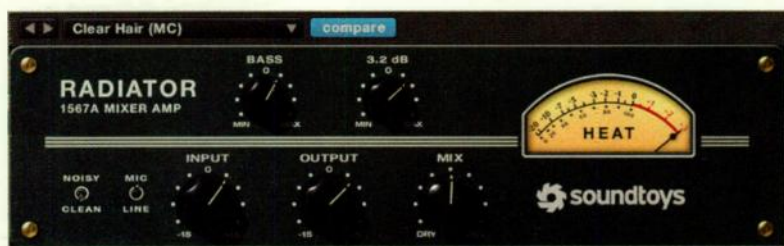
Fig. 3. SoundToys Radiator authentically emulates the sound of a tube mixer, producing tones ranging from subtle saturation to drastic overload.
