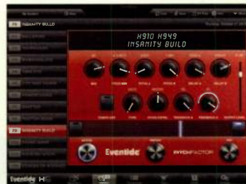
Fig. 1. H9 Control reproduces the front panels of every Eventide stompbox it emulates, with ten knobs and six switches per screen, as well as a ribbon controller. On a computer or iPad, every control appears almost exactly as it does on the original device. On an iPhone, the same controls are split into two vertical screens that you can switch between.
