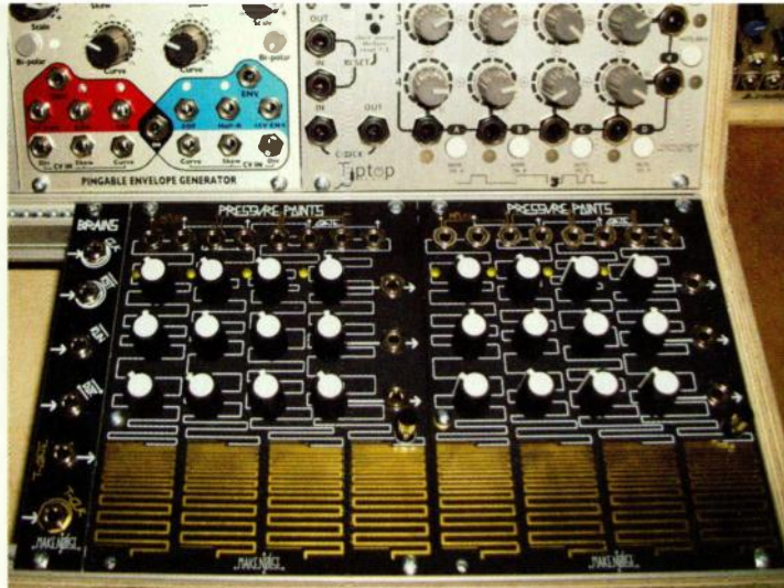
Fig. 2. The two Pressure Points modules in the lower row (built by Make Noise), together with the narrow Brains module to their left, form an eight-step sequencer with touchpads. Above the Pressure Points is a Trigger Riot from Tiptop Audio, a digital module that produces rhythmic trigger/gate signals for analog sequencing.
