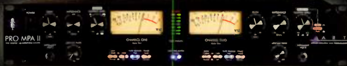
PRO MPA II Two Channel Class-A Tube Mic Preamp TWO CHANNEL TUBE MICROPHONE AMPLIFIER
