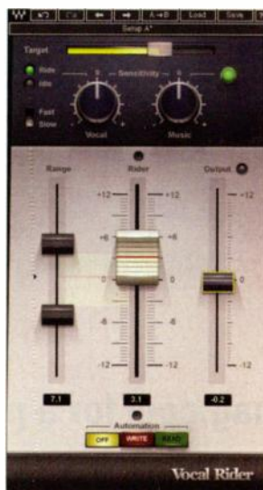
Fig. 2. Waves Vocal Rider dynamically adjusts levels for a vocal track. Here, the plug-in automatically rides an objectionably quiet vocal phrase 3dB higher.
