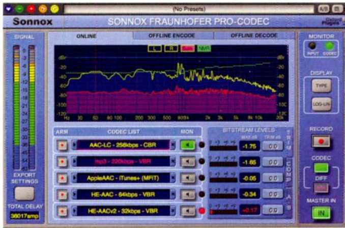
Fig. 3. Sonnox Fraunhofer Pro-Codec offers realtime auditioning of up to five codecs in turn. Here, readouts for the codecs' maximum bitstream levels indicate clipping will occur using the HE-AACv2 codec at the bottom of the list, unless corrected.
