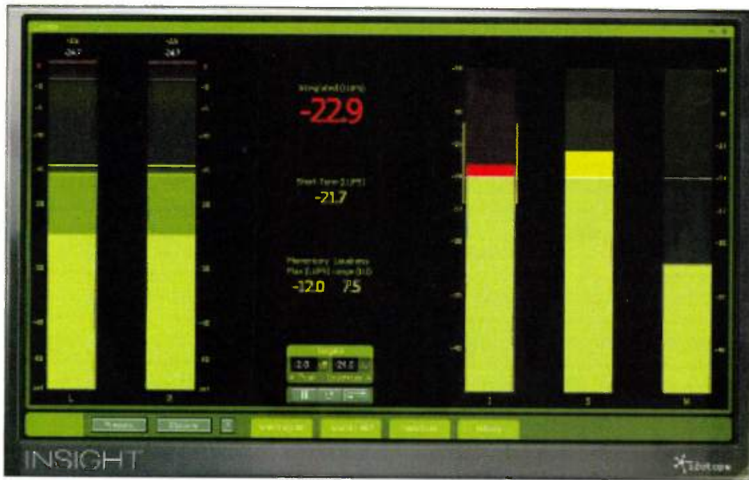
Fig. 2. iZotope Insight's loudness meters indicate program level has exceeded a user-defined -24LUFS loudness target by 1.1 dB, as shown by the numerical readout in the top center of the GUI and the top LEDs in the meter immediately to its right lighting red.
