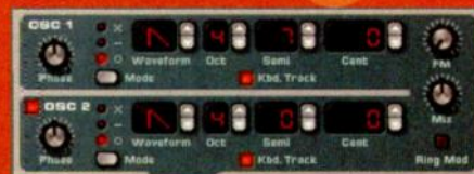
Every two-oscillator synth can re-create the classic electro fifth. Just use sawtooths and tune one oscillator up seven semitones.
