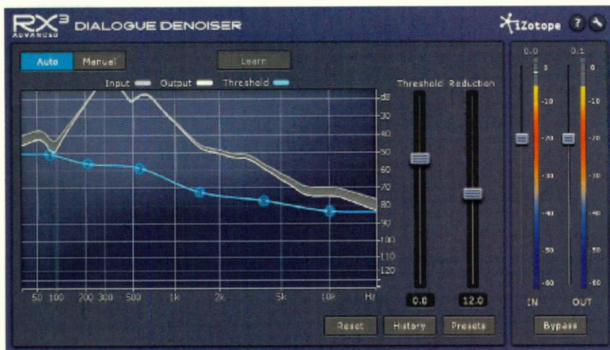
Fig. 1. iZotope RX3 Advanced's Dialogue Denoiser incorporates an all-new adaptive algorithm for ridding tracks of noise. Auto mode is optimized for treating VO tracks.
