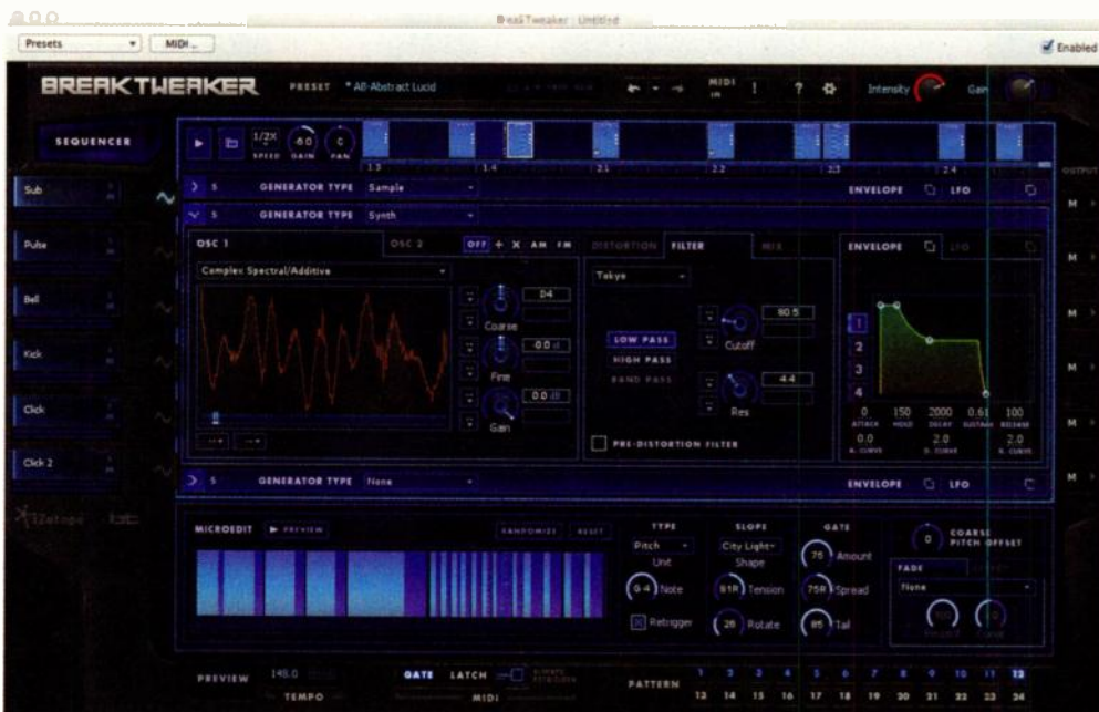
Clicking on the sine-wave graphic next to a track reveals its sample-editing and synthesis parameters for each of its three generators. Each generator can be a sample or a two-oscillator wavetable synth engine.
