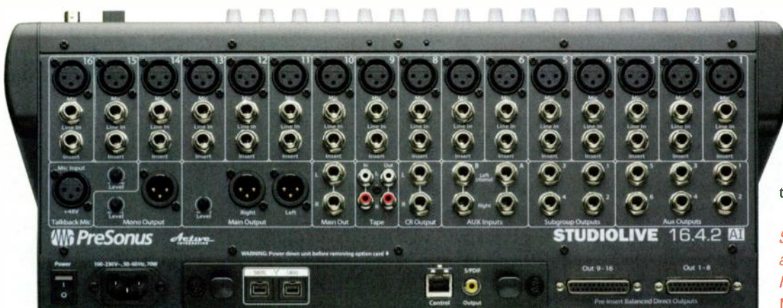
Fig. 1. Each mic input features an XMAX Class A preamp with individually switched phantom power. A card slot is available for FireWire 800, Dante, or Thunderbolt connectivity, while pre-insert balanced direct outputs are available on D-Sub connectors.
