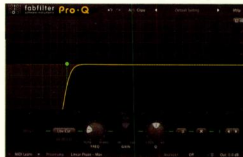
Fig. 2. An HPF is fashioned in FabFilter Pro-Q to suppress vocal pops.
