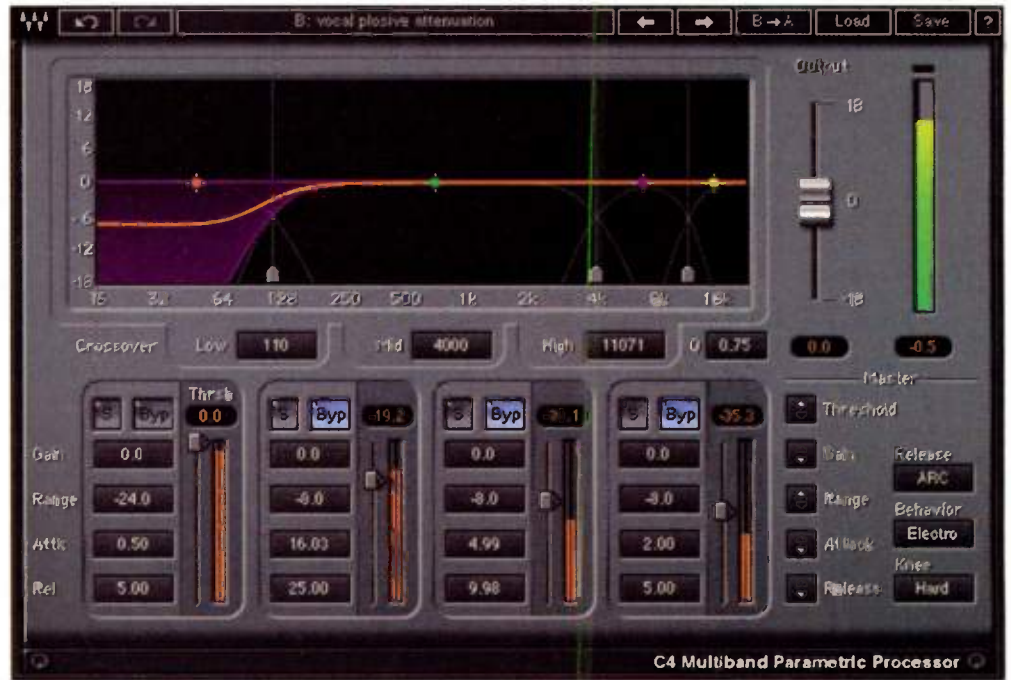
Fig. 3. The Waves C4 plug-in is used to dynamically diminish the effect of vocal pops without thinning the overall timbre of the track.
