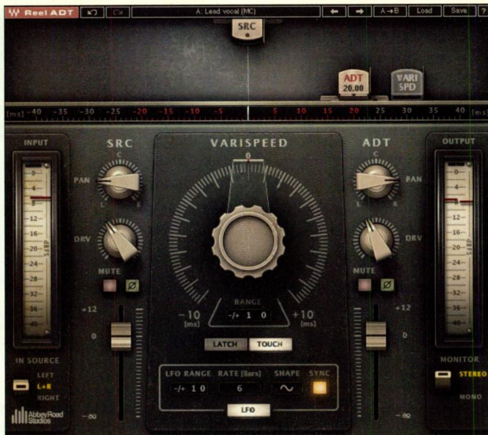
Fig. 1. Waves/Abbey Road Reel ADT provides a Varispeed control that lets you change modulation patterns in real time.
