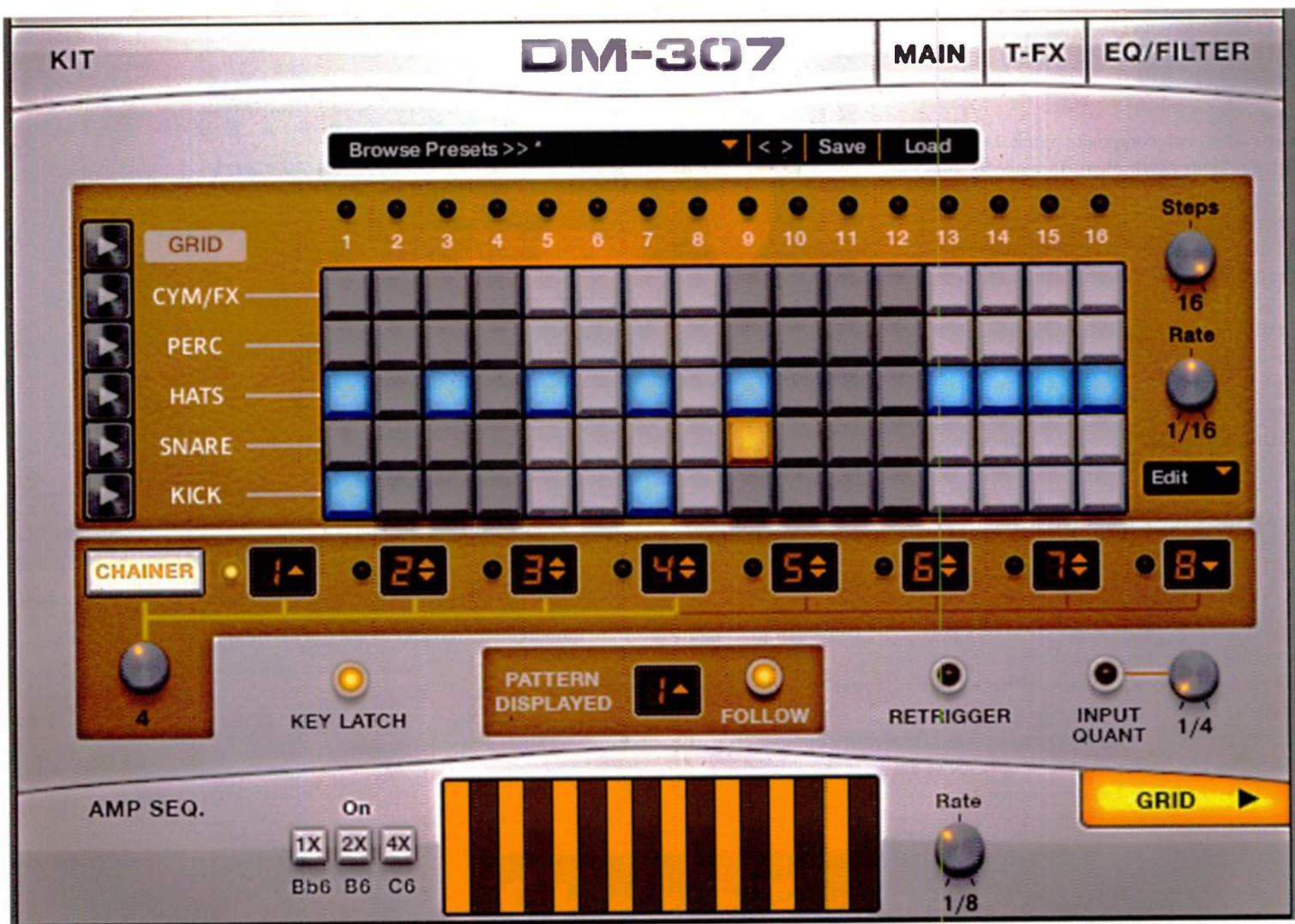
Fig 2. The Grid Window is where most of the pattern sequencing happens. Each of the five banks contains its own sample map.
