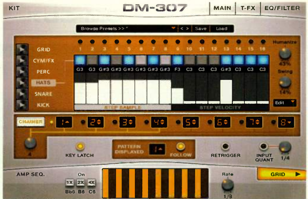
Fig 3. The Step Sample feature lets you trigger different samples attached to a bank's key map. Clicking and dragging the white bar under an event in the sequencer transposes the event, causing it to trigger a different sound (indicated just below the event at the top of the panel).
