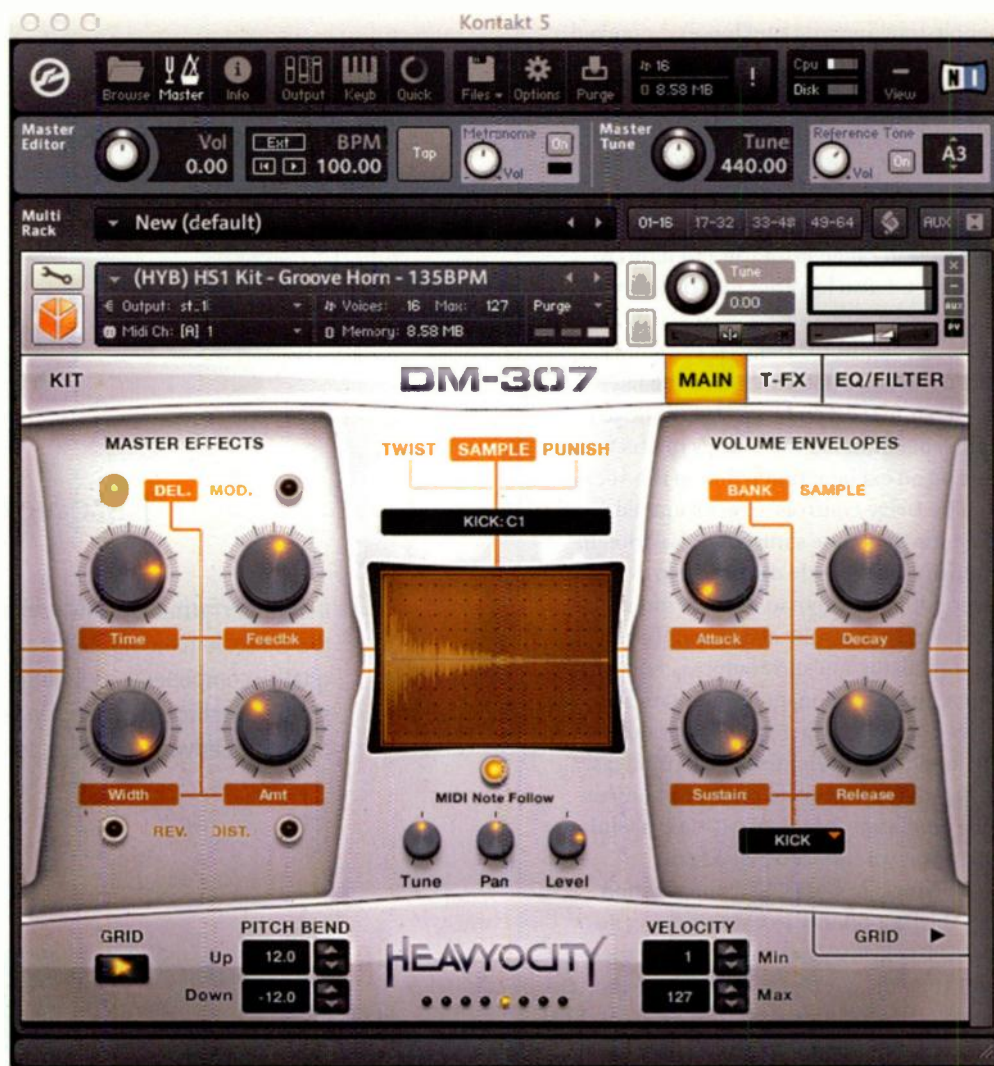
Fig 1. The Main Window is common to all DM-307 patches and grants access to the multieffects, the amp envelope, and Twist and Punish. You can apply the amp envelope to individual sounds on the patch key map.
