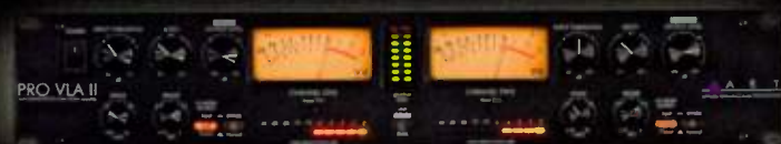
PRO VLA II Two Channel VCA-less Vactrol Opto Tube Compressor Compressor / Leveling Amplifier
