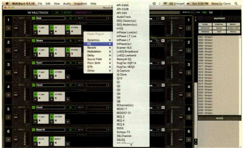
Fig. 1. Six racks added to a MultiRack session. Each rack has independent audio I/O and plug-ins that are accessed by clicking the + symbol in the rack. The open plug-in menu displays available EQs.
