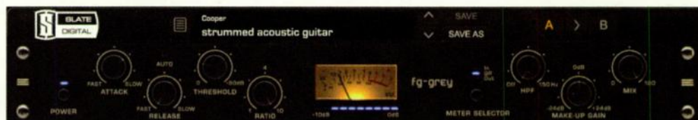
Fig. 2. Slate Digital FG-Grey convincingly emulates the compression curve produced by an SSL 4000 Series bus compressor.
