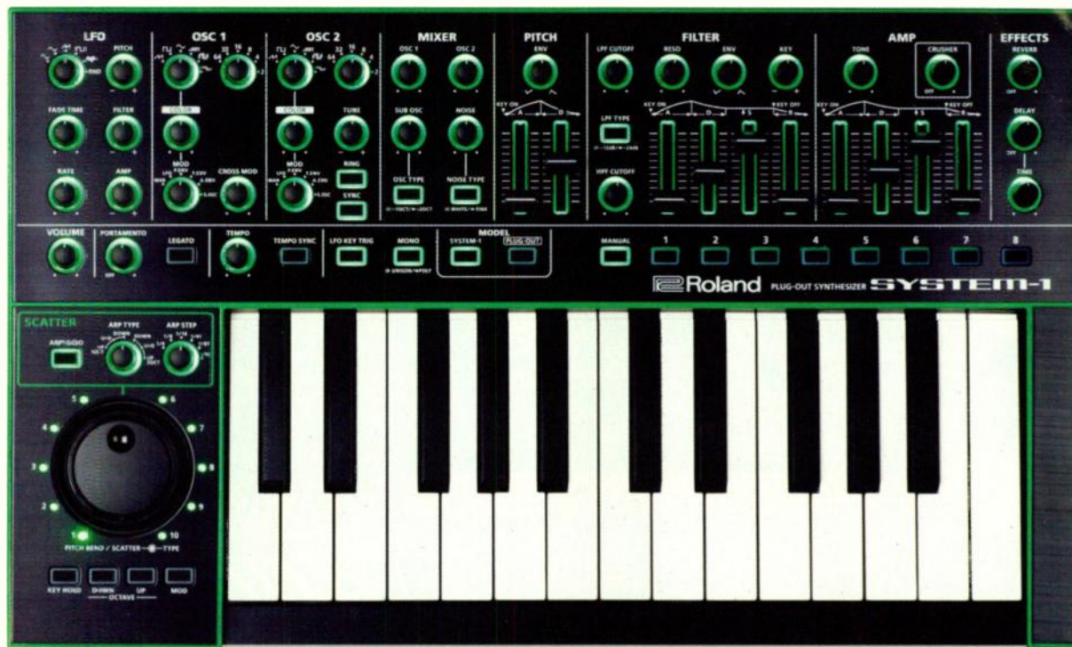
Fig. 1. Everything you need to modify a sound is immediately available on the front panel. When you twist the Scatter dial to vary the arpeggio, the System-1's green LED backlights blink to show you which, if any, parameters have changed.
