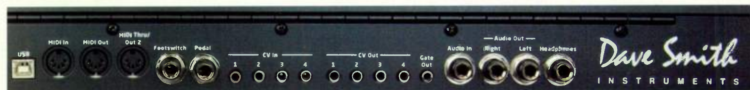
Fig. 3. If you have other instruments or modules with control-voltage connections, the Pro 2 lets you assign any CV input to any destination and any source to any CV output. It can scale and invert control voltages in either direction.
