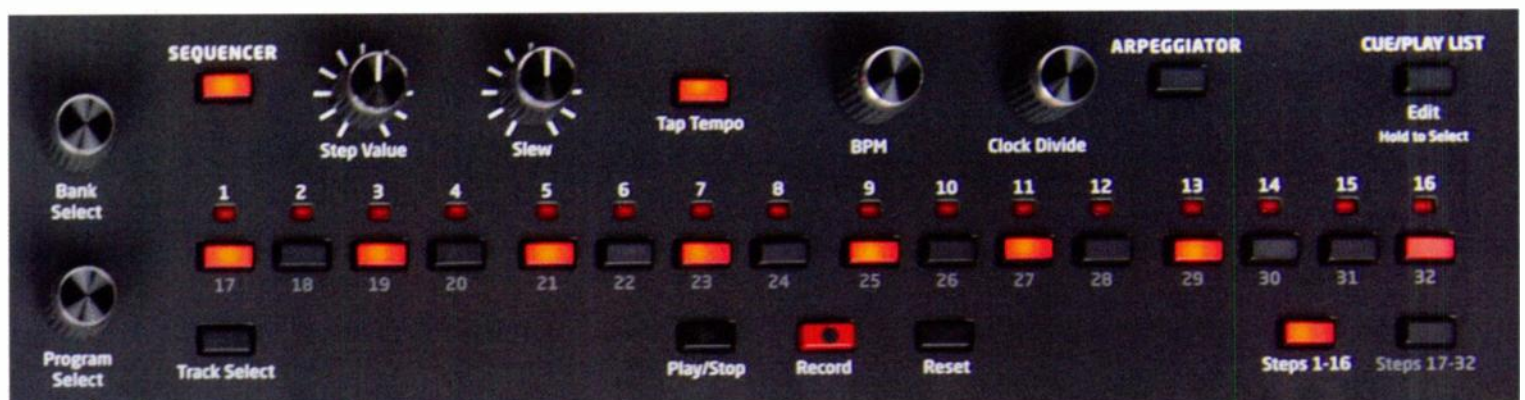
Fig. 4. The refined step sequencer gives you as many as 31 tracks that serve as independent modulation sources, enabling performance capabilities that would be impossible on most synths.
