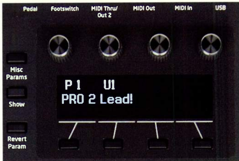
Fig. 2. Four rotary encoders and four buttons control whatever parameters are displayed in the OLED.
