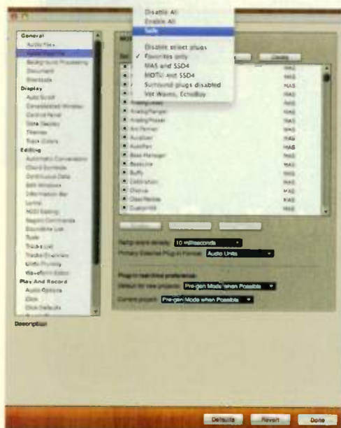
Fig. 1. To disable all third-party plug-ins in DP, open the Audio Plug-ins preference pane in Digital Performer's Preferences window and select Safe in the Plug-in Sets drop-down menu.
