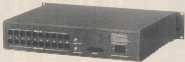
The rear panel of the MIDIBUDDY MMP shown here with optional SCSI port.
