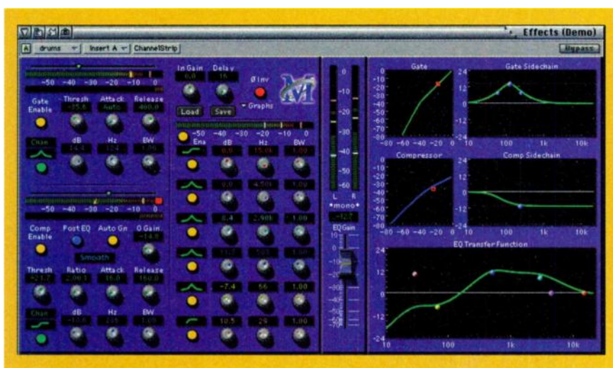
FIG. 1: Controls and metering for ChannelStrip 's processing blocks are organized on the left side of the window. On the right side, interactive graphs depict the action of each processor and offer additional parameter control points that you can drag to edit settings.
