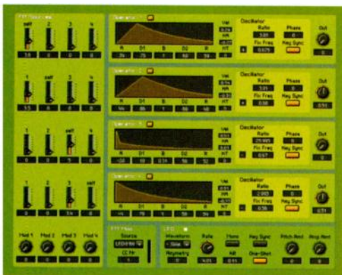
The FM4 Ensemble in Native Instruments Reaktor 5.1 uses four operators, each of which has its own envelope. The modulation matrix (which functions like the matrix in Fig. 1) is on the left.
