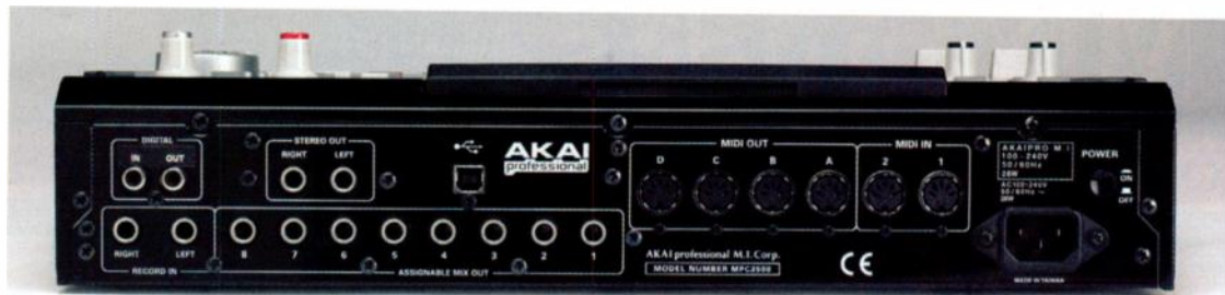
FIG. 2: The MPC2500's rear panel sports a generous complement of inputs and outputs. In addition to stereo analog ins and outs, you get eight assignable analog outs, coaxial S/PDIF I/O, two merged MIDI Ins, and four independent MIDI Outs.
