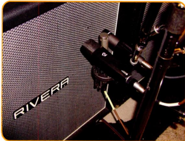
FIG. 1: Like many engineers, Ross Hogarth combines several different mics on an electric guitar speaker to create a tone to match a particular song. His typical setup includes (left to right) a Sennheiser 421, a Royer R-121, and a Shure SM57.
