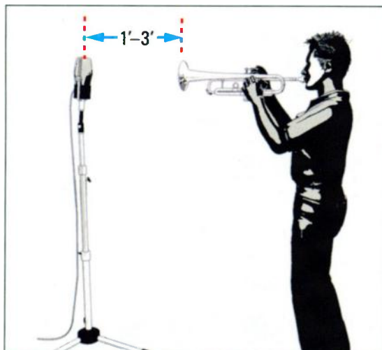
FIG. 8: Eddie Kramer extols the sound of a trumpet recorded with an RCA 44 at approximately 2 feet. Each engineer offered his own preferences for distance between mic and musician, but the room sound and volume of the musical passage must also be taken into consideration.
