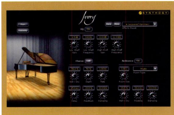
FIG. 2: Ambience, Chorus, and 2-band EQ are available on Ivory's Effects screen, which also lets you load and save groups of effects presets.
