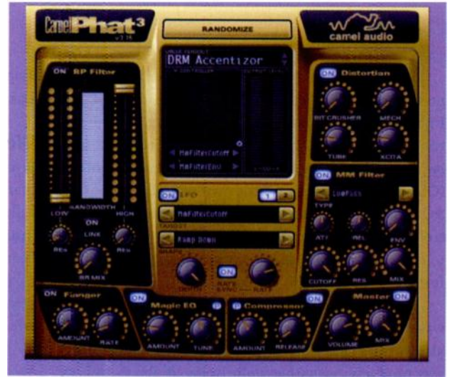
FIG. 1: CamelPhat's control panel layout mirrors the signal flow from BP Filter (top left) to the master output (bottom right).
