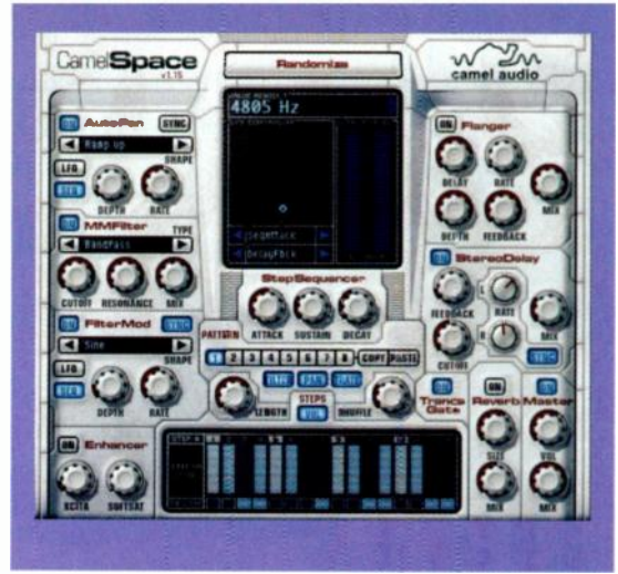
FIG. 2: CamelSpace's step sequencer (bottom center) can control the Trance Gate, the AutoPan position, and the filter cutoff.
