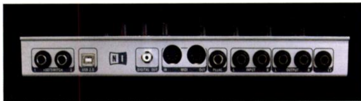
FIG. 4: Kore's rear panel houses jacks for audio, MIDI, hardware controllers, and S/PDIF.
