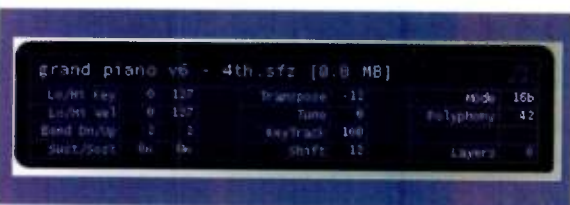
FIG. 1: Set the Shift and Transpose parameters in Dimension Pro's Multisample window to equal but opposite values to create pitch-shifted timbres.
