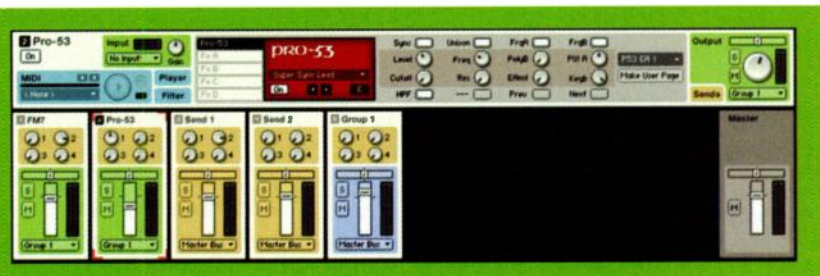
FIG. 1: There are three views of the KoreSound mixer: Rack, Mixer, and Combined (shown here).
