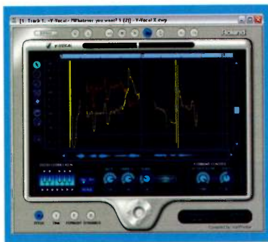
FIG. 5: V-Vocal is the first appearance of Roland's VariPhrase technology in a digital audio sequencer, Cakewalk Sonar 5 Producer Edition. Because it isn't a plug-in, V-Vocal lets you resize its window using normal Windows techniques.
