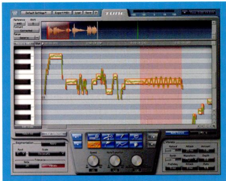
FIG. 10: Waves Tune is a multiformat plug-in that can scan and manipulate pitch and tempo for tracks as long as ten minutes. Pitch changes appear as a series of blocks and curves.
