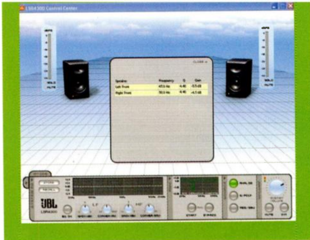
FIG. 3: The Control Center software gives you finer control over levels, input switching, EQ, muting, and more. It also displays the specific parameters of the RMC EQ curves (as shown here) that the system has generated.
