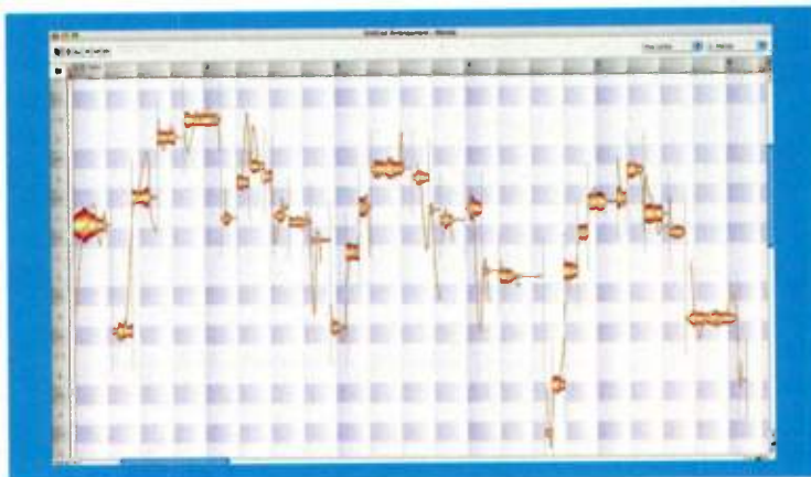
FIG. 6: Celemony Melodyne displays audio events as Blobs on a grid and lets you manipulate them as if they were MIDI events.
