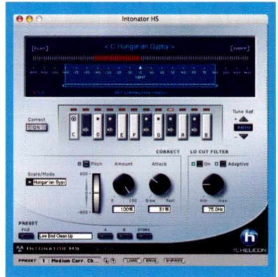
FIG. 8: TC-Helicon Intonator HS transposes pitch so it matches whatever scale you select. Presets include chromatic, major, minor harmonic, Mixolydian, Hawaiian, Javanese Pelog, and more than 40 others.
