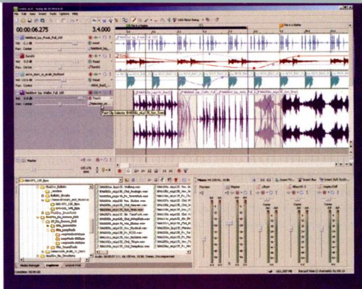
FIG. 1: Acid's main screen includes a file browser and database display (bottom left) and a mixer (bottom right). The lower area can be resized to show more tracks. Note the in-line display of track envelope data and the crossfade between overlapping clips.
