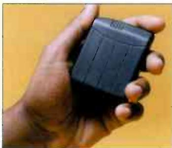
Based on defense industry technology, this meter is kept with each respondent as they go about their daily routine. Each station's signal will include a silent, unique encoding that allows PPM to know and
