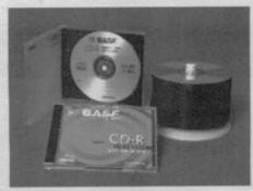
The Recordable Compact Disc (CD-R) is a write-once optical disc. Digital audio or computer data is recorded on the disc by laser, rendering it equivalent to a mass produced CD or CD-Rom.
