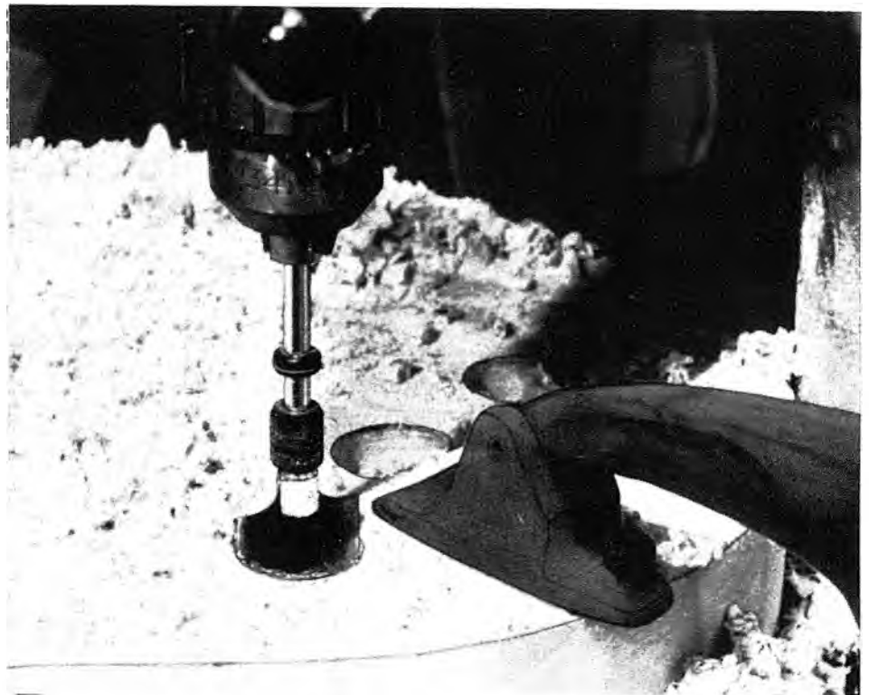
It is essential to use a secure clamp when drilling with a 'Flat-bit'.
