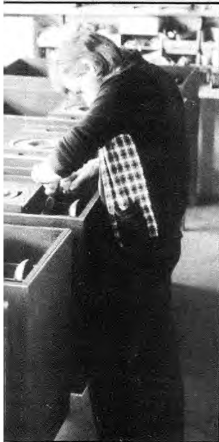
Assembly of radial horn units for Century IV
