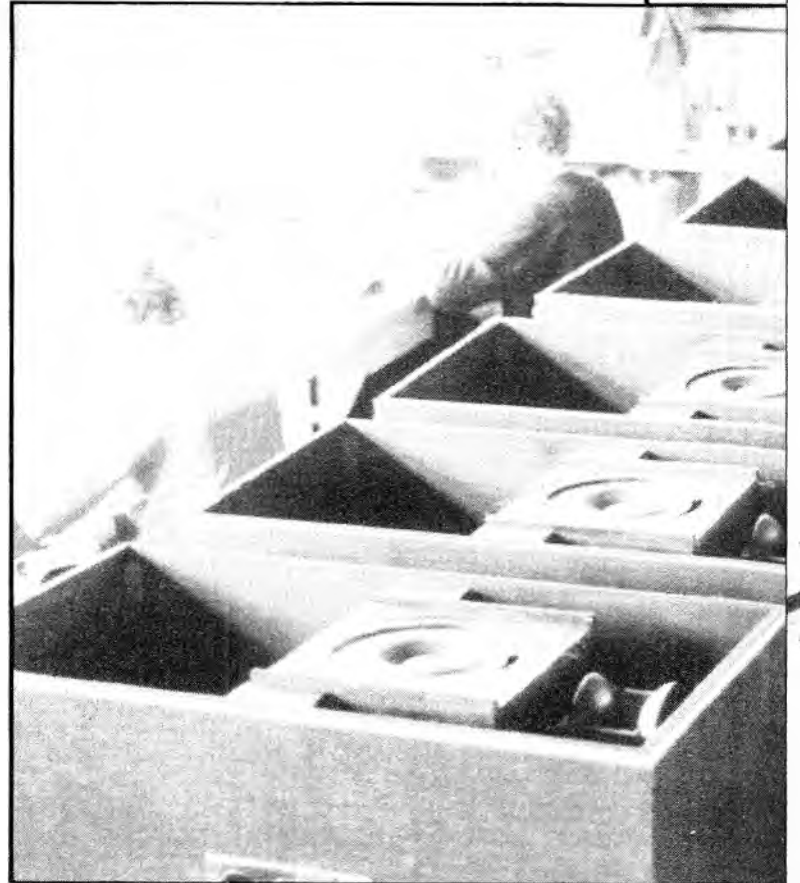
Assembly of Eliminator 10s. The drive units visible are the ST350/A H.F. Horn and the new vented midrange unit
